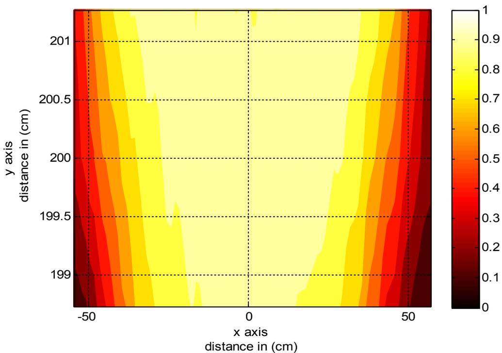
Figure 38: Spatial correlation at 3.1 – 10.6 GHz with antennas orientated vertically, first 3 nanoseconds of the received signal.
