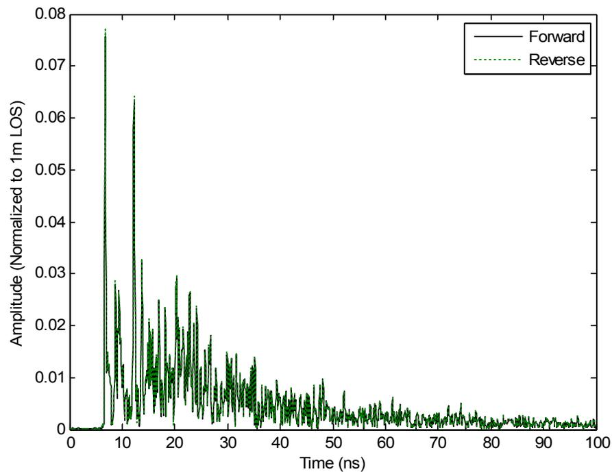
Figure 13: NLOS reciprocity at scenario 2 with horizontal polarized antennas, and the lab and office antenna heights are at a 1.0 meter elevation.
