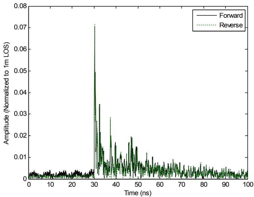
Figure 11: NLOS reciprocity at scenario 5 with vertical polarized antennas separated by 10 meters with an elevation of 1.0 meter.
