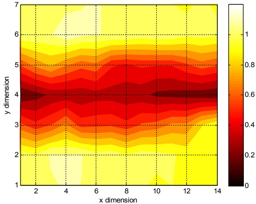
Figure 29: Normalized power coefficient for body shadowing, in scenario 1 with a frequency bandwidth of 3.1 – 10.6 GHz and the antennas orientated vertically.
