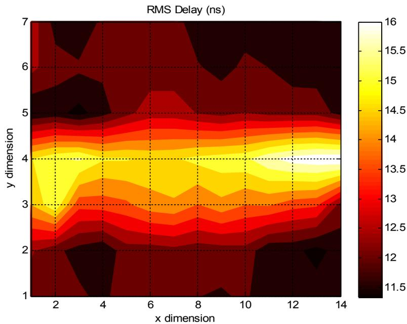
Figure 33: RMS delay spread with body shadowing in scenario 6 with a frequency bandwidth of 3.1 – 10.6 GHz and the antennas orientated vertically.
