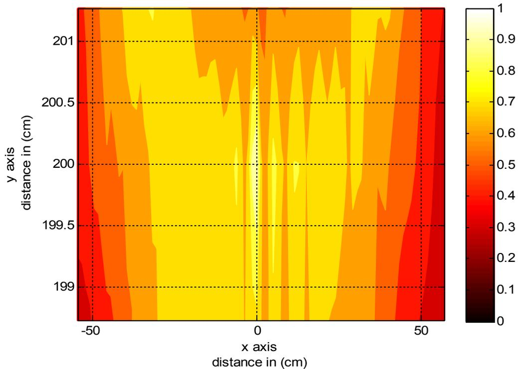
Figure 35: Spatial correlation at 3.1 – 10.6 GHz with antennas orientated vertically, total received signal.
