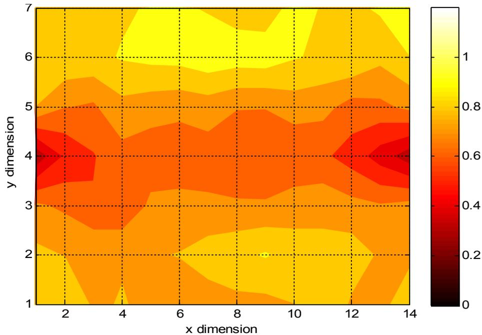
Figure 27: Normalized power coefficient for body shadowing, in scenario 1 with a frequency bandwidth of 0.38 – 3.8 GHz and the antennas orientated horizontally.
