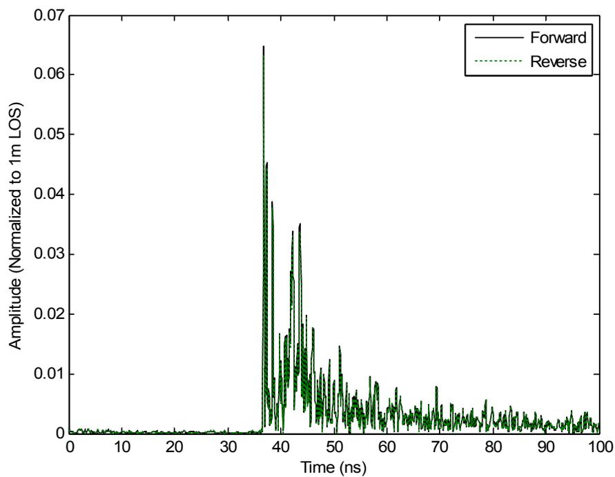
Figure 19: NLOS reciprocity at scenario 4 with horizontal polarized antennas separated by 12 meters with an elevation of 1.0 meters.
