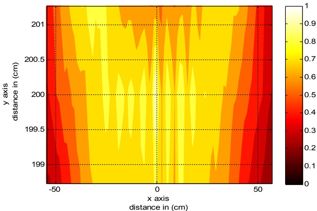
Figure 36: Spatial correlation at 3.1 – 10.6 GHz with antennas orientated vertically, first 20 nanoseconds of the received signal.
