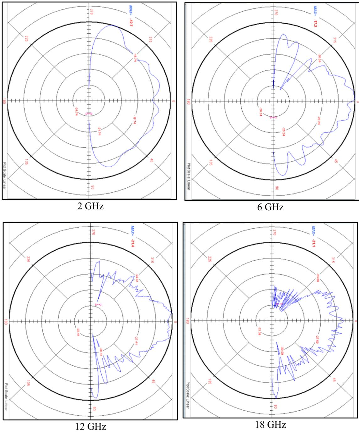
Figure 41: EM-6865 Elevation Patterns
