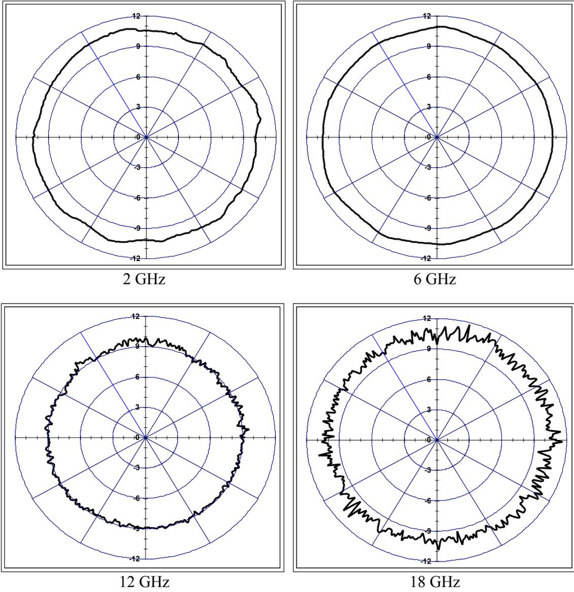
Figure 40: EM-6865 Azimuth Patterns
