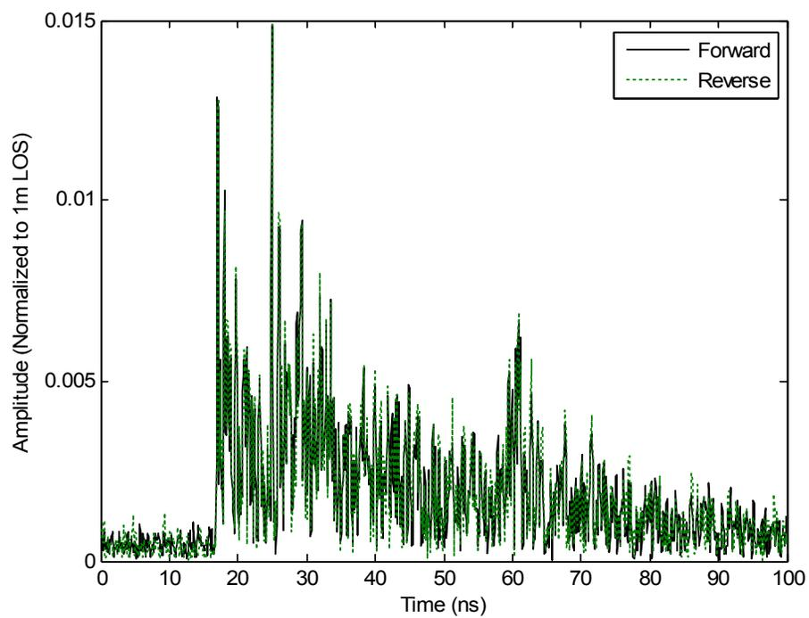
Figure 9: NLOS reciprocity at scenario 3 with vertical polarized antennas, and the lobby and office antenna heights at a 1.5 and 1.0 meter elevation, respectively.
