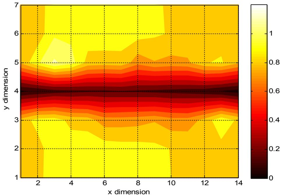
Figure 30: Normalized power coefficient for body shadowing, in scenario 1 with a frequency bandwidth of 3.1 – 10.6 GHz and the antennas orientated horizontally.
