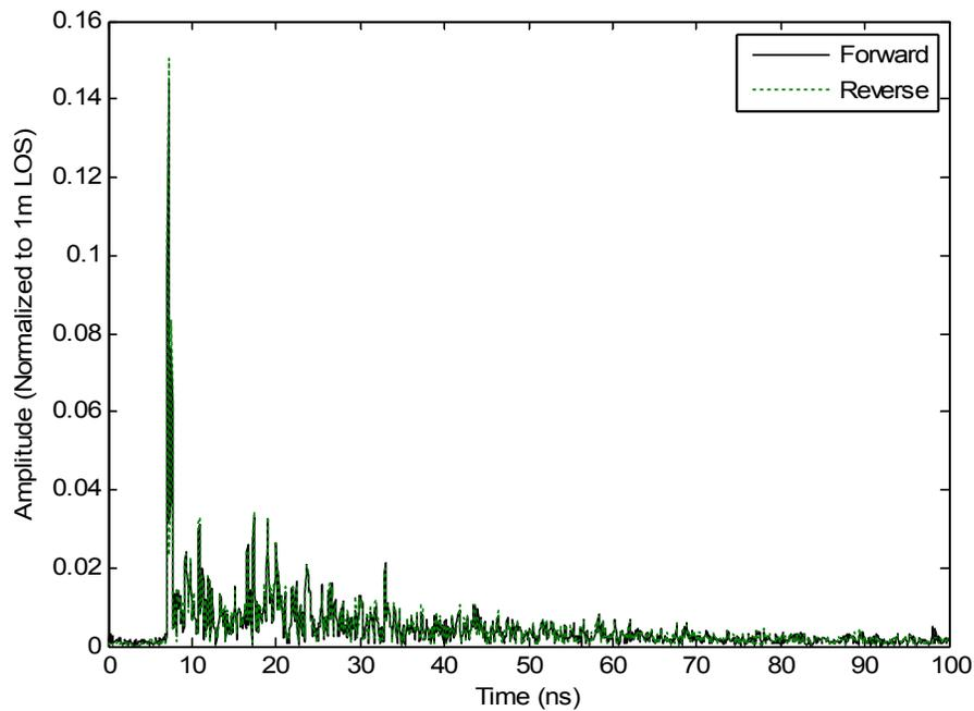
Figure 7: NLOS reciprocity at scenario 2 with vertical polarized antennas, and the lab and office antenna heights at 1.0 and 2.0 meter elevation respectively.
