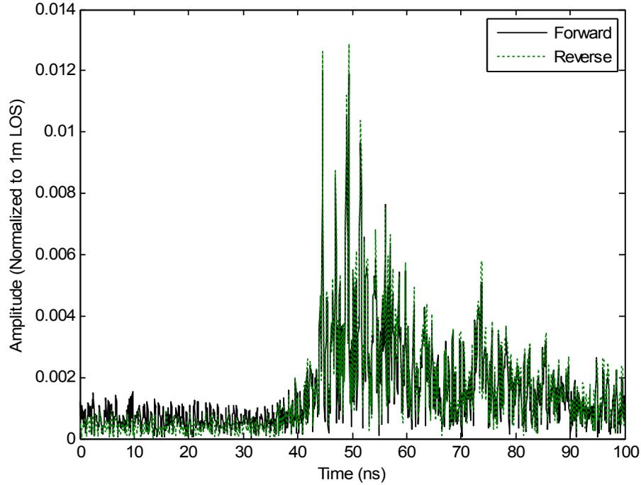
Figure 12: NLOS reciprocity at scenario 5 down the hallway and around the corner with vertical polarized antennas separated by 10 + 3 meters with an elevation of 1.0 meter.
