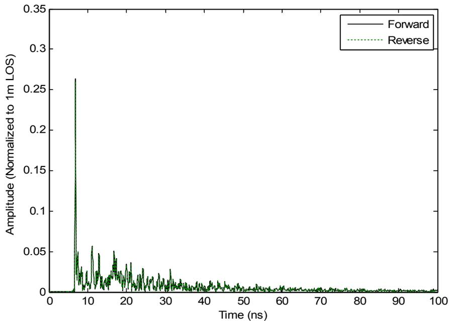
Figure 14: NLOS reciprocity at scenario 2 with horizontal polarized antennas, and the lab and office antenna heights at 1.0 and 1.4 meter elevation, respectively.
