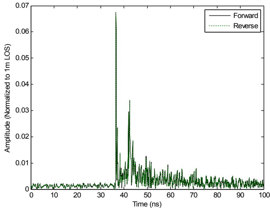
Figure 10: NLOS reciprocity at scenario 4 with vertical polarized antennas separated by 12 meters with an elevation of 1.0 meter.
