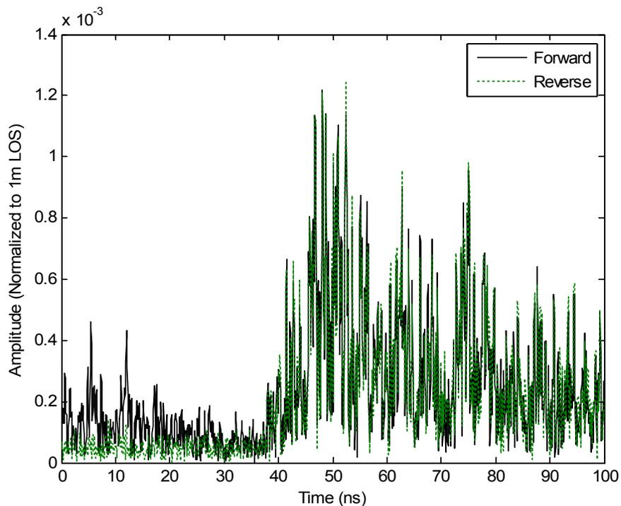
Figure 22: NLOS reciprocity at scenario 5 down the hallway and around the corner with horizontal polarized antennas along the x, y axis separated by  $10 + 3$  m with an elevation of 1 m.
