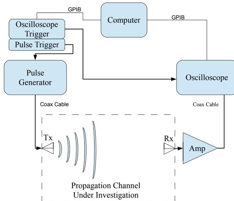
**Figure 1:** Block diagram of the time domain setup.
