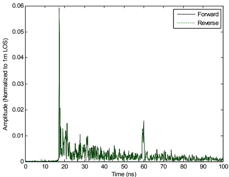
Figure 18: NLOS reciprocity at scenario 3 with horizontal polarized antennas, and the lobby and office antenna heights at a 1.8 and 1.0 meter elevation, respectively.
