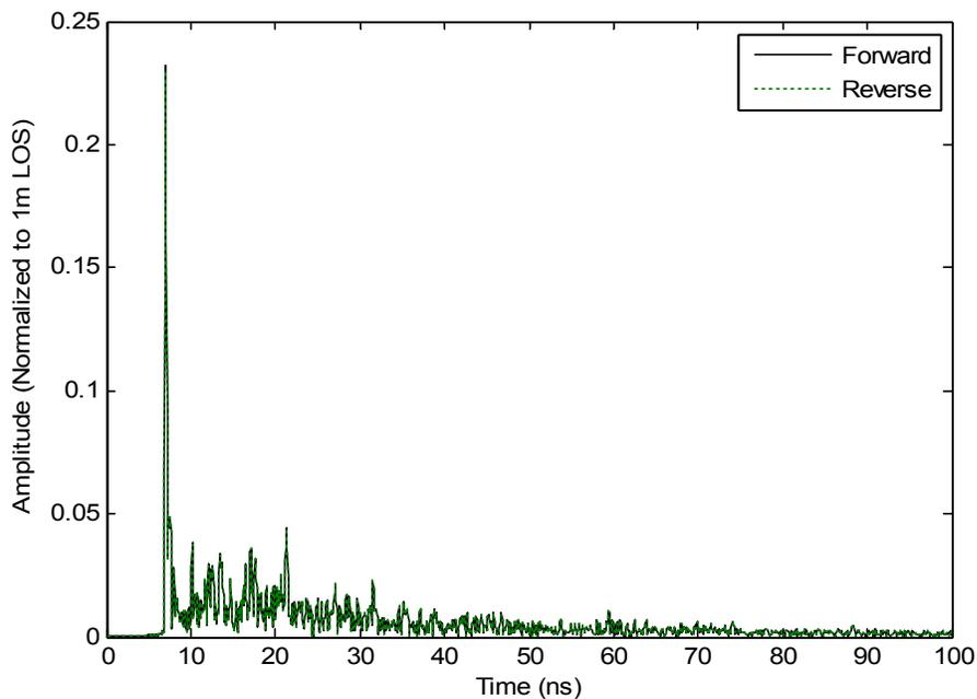
Figure 15: NLOS reciprocity at scenario 2 with horizontal polarized antennas, and the lab and office antenna heights at 1.0 and 1.8 meter elevation, respectively.
