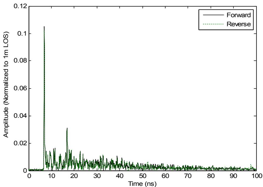
Figure 5: NLOS reciprocity at scenario 2 with vertical polarized antennas, and the lab and office antenna heights are at a 1.0 meter elevation.
