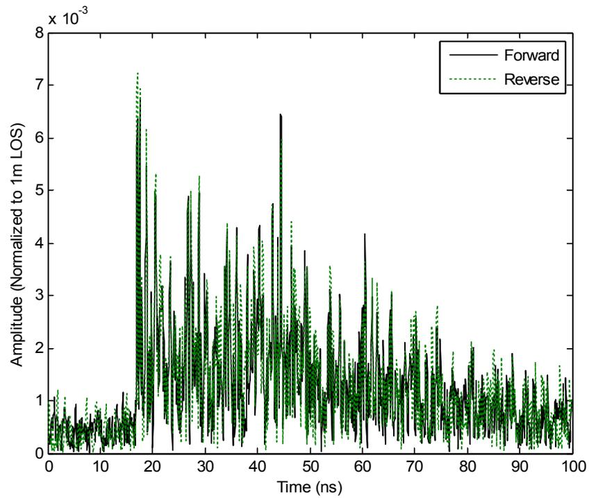
Figure 8: NLOS reciprocity at scenario 3 with vertical polarized antennas, and the lobby and office antenna heights are at a 1.0 meter elevation.
