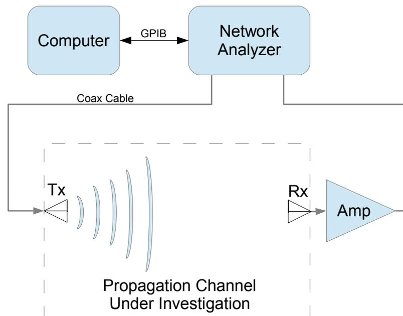
**Figure 3:** Block diagram of the frequency domain setup.
