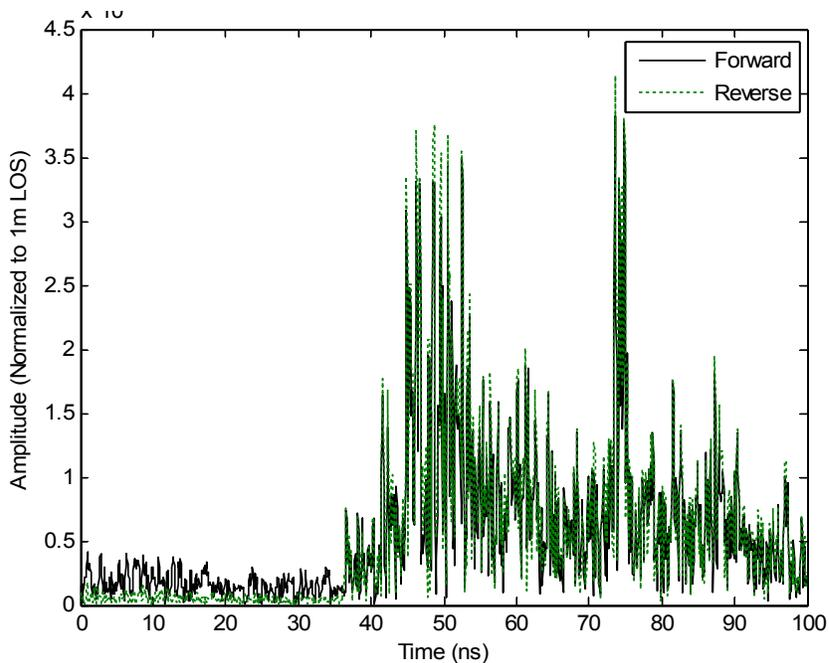
Figure 21: NLOS reciprocity at scenario 5 down the hallway and around the corner with horizontal polarized antennas separated by  $10 + 3$  m with an elevation of 1 m.
