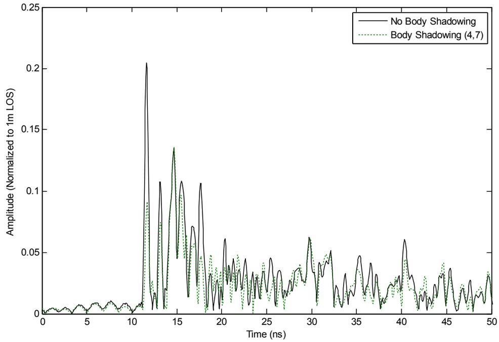
Figure 26: Correlation with and without body shadowing in scenario 1 of the received signal, with a bandwidth of 0.38 – 3.8 GHz and the antennas orientated horizontally.
