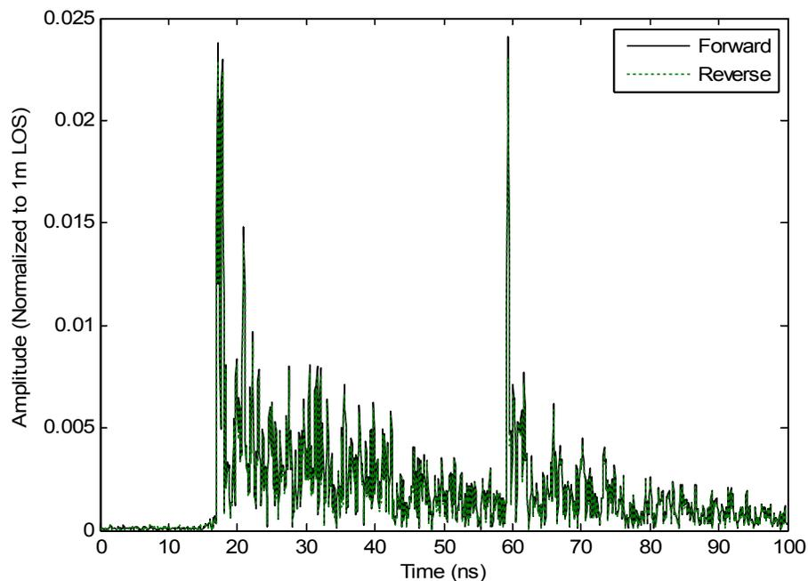
Figure 17: NLOS reciprocity at scenario 3 with horizontal polarized antennas, and the lobby and office antenna heights at a 1.4 and 1.0 meter elevation, respectively.
