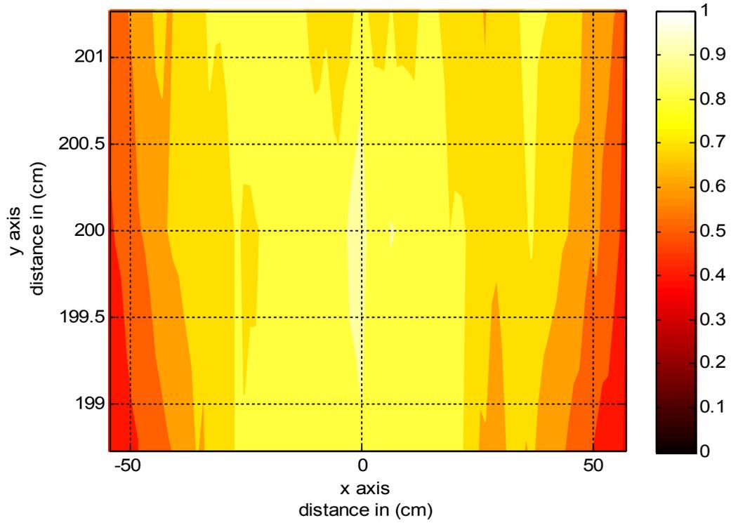
Figure 39: Spatial correlation at 3.1 – 10.6 GHz with antennas orientated horizontally, total received signal.
