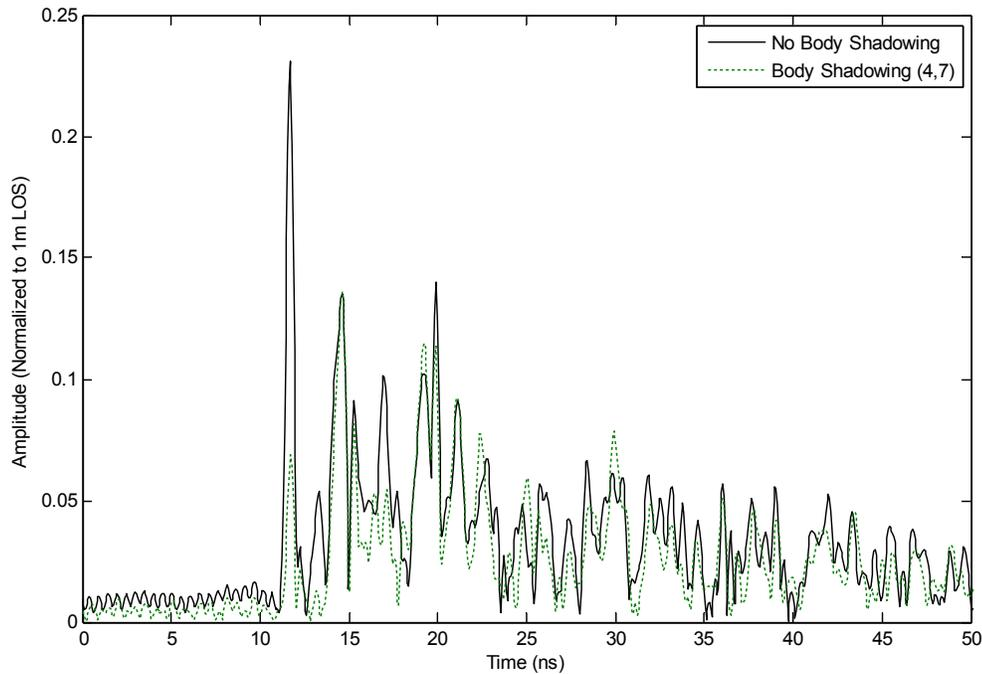
Figure 24: Correlation with and without body shadowing in scenario 1 of the received signal, with a bandwidth of 0.38 – 3.8 GHz and the antennas orientated vertically.
