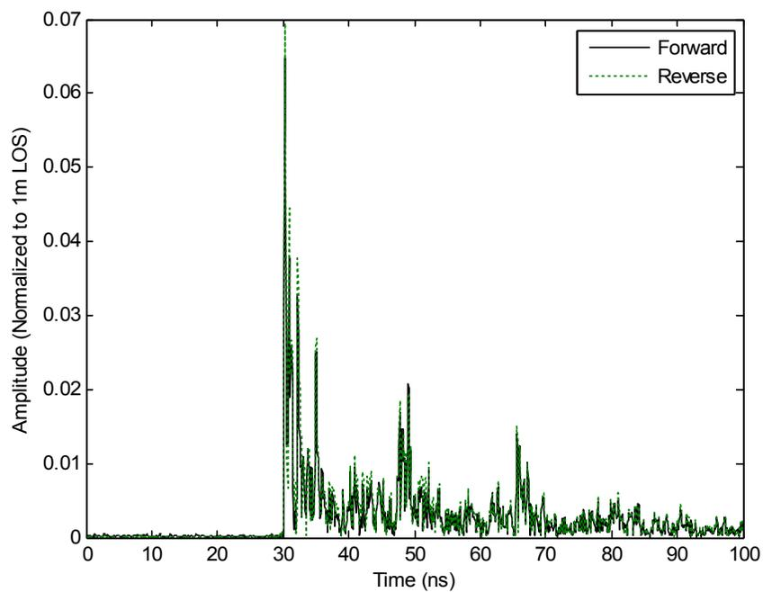
Figure 20: NLOS reciprocity at scenario 5 with horizontal polarized antennas separated by 10 meters with an elevation of 1.0 meters.
