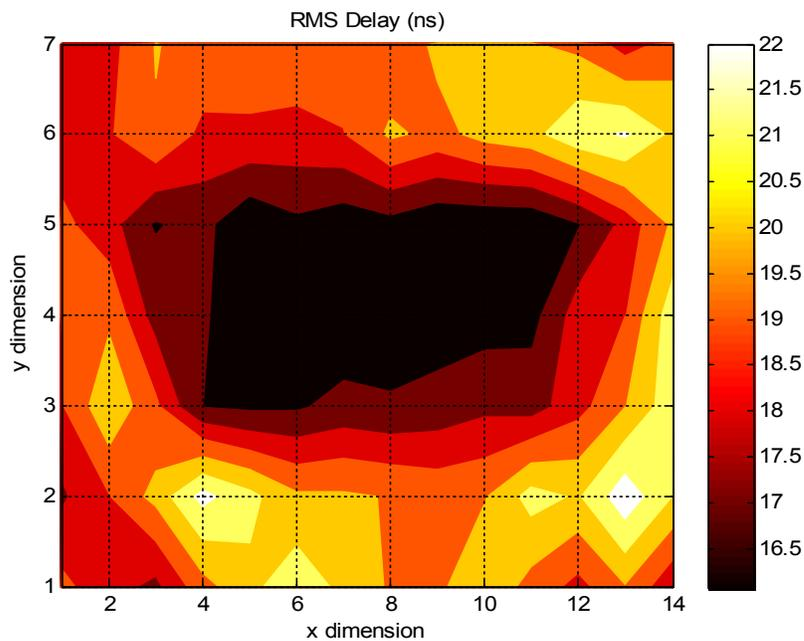
Figure 31: RMS delay spread with body shadowing in scenario 1 with a frequency bandwidth of 0.38 – 3.8 GHz and the antennas orientated vertically.
