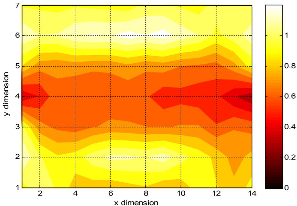
Figure 25: Normalized power coefficient for body shadowing in scenario 1 with a frequency bandwidth of 0.38 – 3.8 GHz and the antennas orientated vertically.
