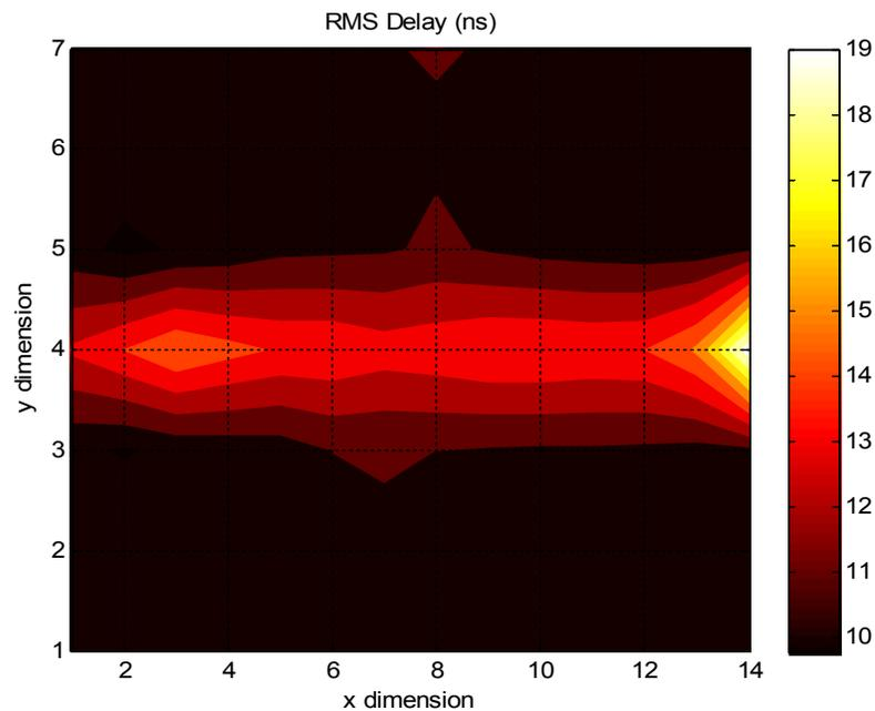
Figure 34: RMS delay spread with body shadowing in scenario 6 with a frequency bandwidth of 3.1 – 10.6 GHz and the antennas orientated horizontally.
