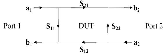
**Figure 2:** Block diagram of S-parameters
