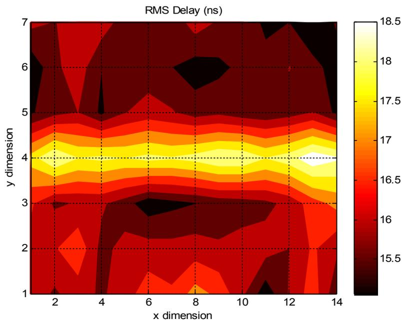
Figure 32: RMS delay spread with body shadowing in scenario 1 with a frequency bandwidth of 0.38 – 3.8 GHz and the antennas orientated horizontally.
