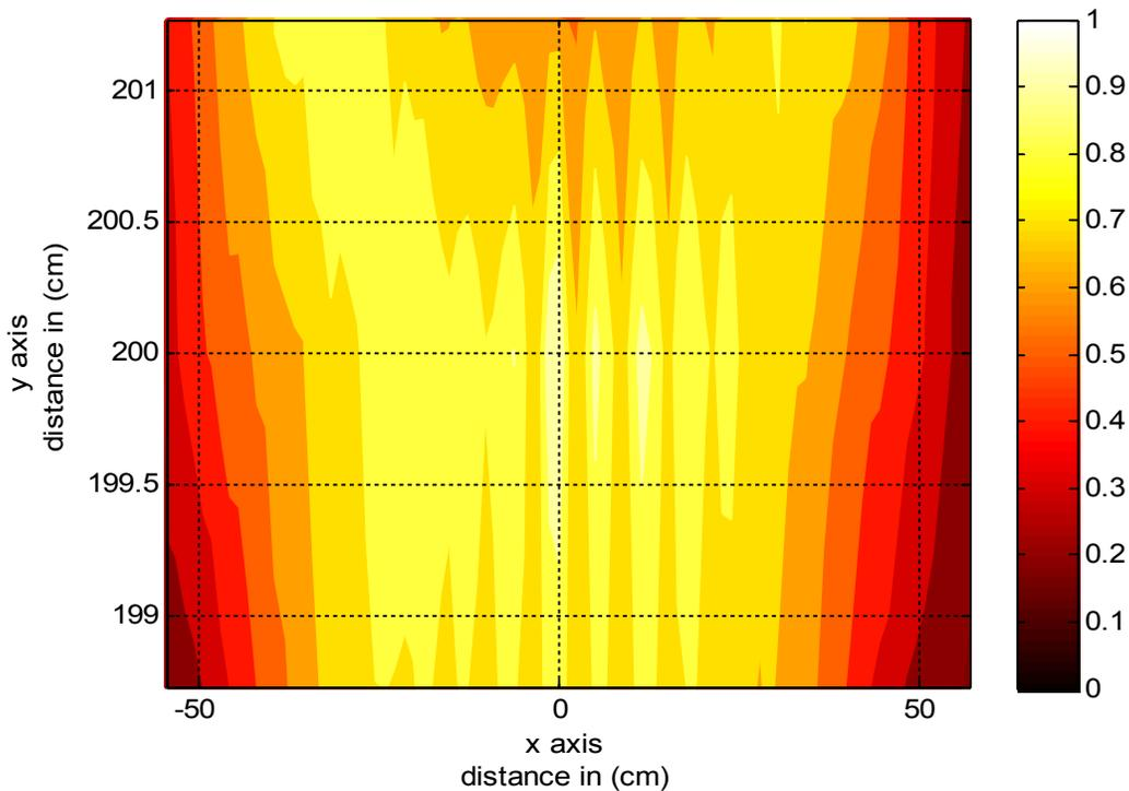
Figure 37: Spatial correlation at 3.1 – 10.6 GHz with antennas orientated vertically, first 10 nanoseconds of the received signal.
