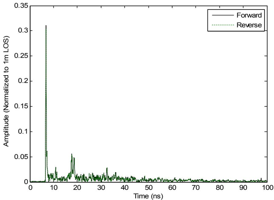
Figure 6: NLOS reciprocity at scenario 2 with vertical polarized antennas, and the lab and office antenna heights at 1.0 and 1.4 meter elevation, respectively.
