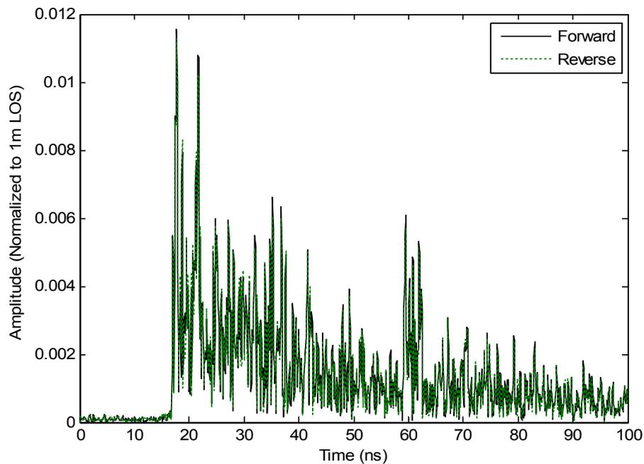
Figure 16: NLOS reciprocity at scenario 3 with horizontal polarized antennas, and the lobby and office antenna heights are at a 1.0 meter elevation.
