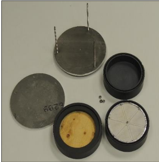
Figure 3 - Modified cup disassemble parts
