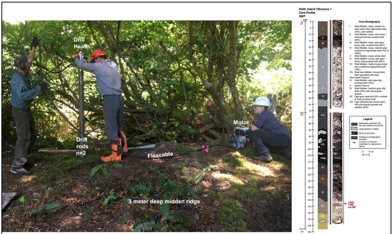
Figure 1. Right: Vibracoring at Kakmakimilth (Photo: Iain McKechnie). Left: Keith Island 1 profile drawing, GSC core photograph, radiocarbon sample locations and date ranges (cal BP) and description of core stratigraphy.
