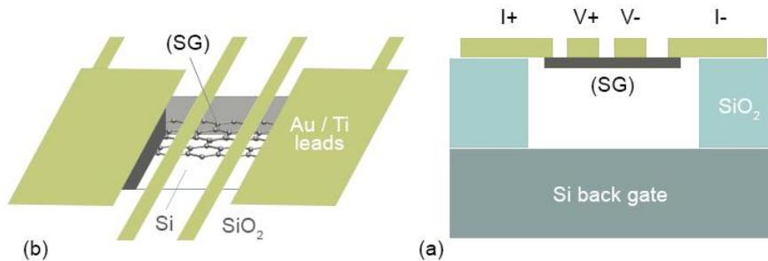
Figure 2. A suspended graphene (SG) sample. (a) Schematic representation of the structure of the SG devices (side view). (b) top view. The electrodes are shown in yellow.
