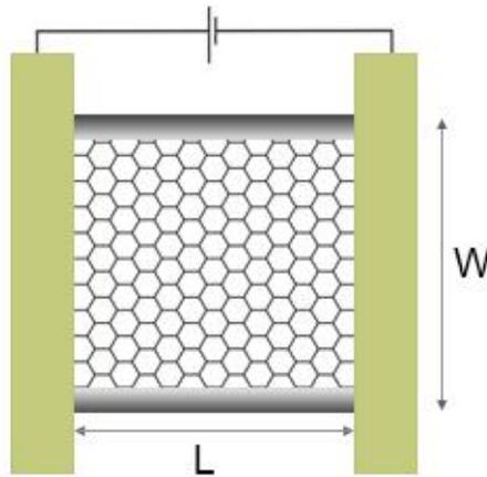
Figure 3. Schematic of a strip of graphene of width  $W$ , with two electrodes (yellow rectangles) separated by a distance  $L$ . A voltage source creates a current through the strip.
