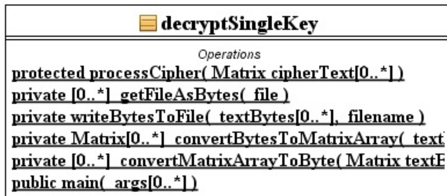
Figure 4.7: UML class diagram of the decryptSingleKey class
