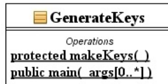
Figure 4.8: UML class diagram of the GenerateKeys class
