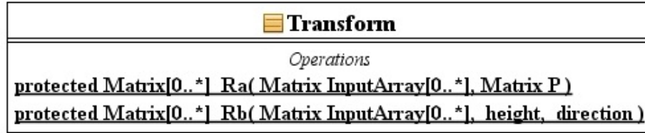
Figure 4.2: UML class diagram of the Transform class
