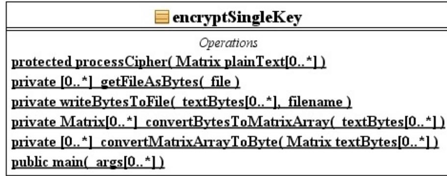
Figure 4.6: UML class diagram of the encryptSingleKey class
