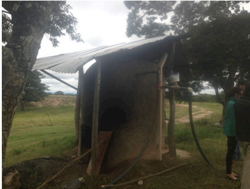
Photo 5.34: Furnace constructed to heat ponds
