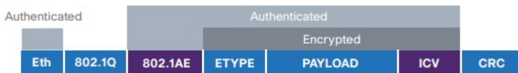
Figure 2.5: Unencrypted VLAN tag in a MACsec encrypted frame [4].
