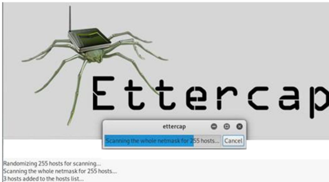
Figure 4.24: MITM attacker scanning the subnet for hosts to target.
