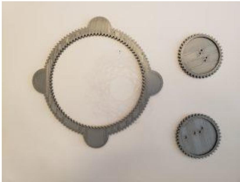
In Figure 7, two copies of the fully printed shape from Figure 5 and 6 are displayed along with their 3D printed counterpart. These objects were printed with Poly-Lactic Acid (PLA) plastic, a durable, non-toxic, and beginner-friendly material. Looking closely, one can see striations on the objects, a result of the of how the strands of plastic are thinly layered and deposited by the printer nozzle.
