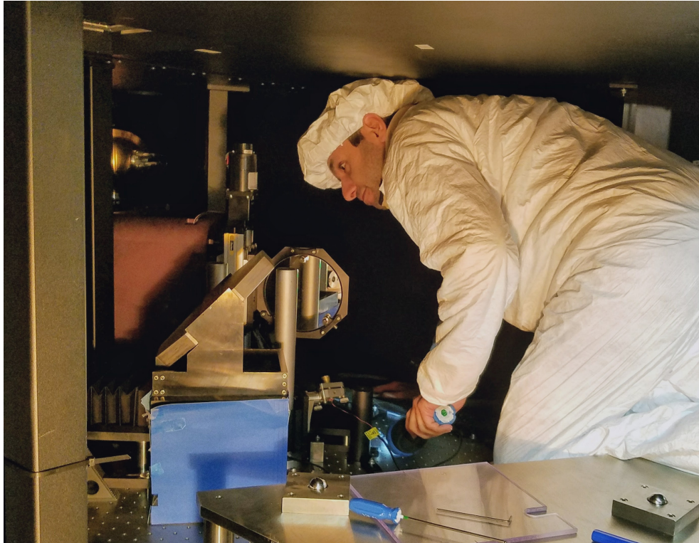
Figure 2.23: During the replacement procedure, the author carefully crawling in the confined space of the Keck 2 AO bench positioned on the Nasmyth focus of the telescope, preparing alignment setup ready to remove ISM.
