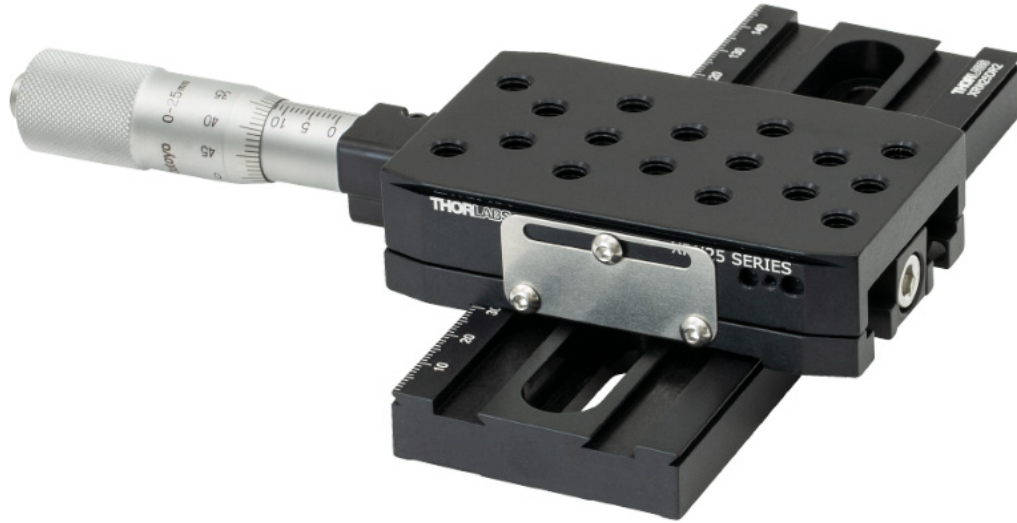
Figure 3.26: The 2" wide dovetail rails and compact quick connect linear stages. The stage can only move along the rail which makes the alignment of each arm considerably simpler compared to using the traditional free-to-place stages for this application.
