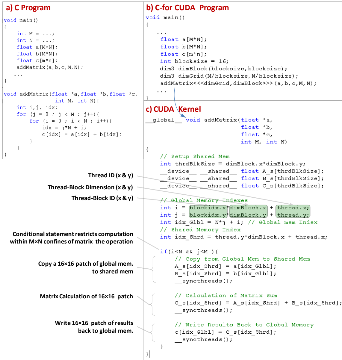
Figure 3.6: Programming sample of the matrix operation (C=A+B). (a) sample nested loop algorithm done in C.(b) The same matrix operation implemented in C-for-CUDA which launches (c) the kernel code on the GPU.
