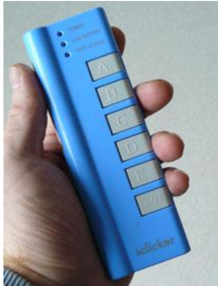
Figure 3: an iClicker classroom response unit, which communicates via radio signals to a base station
