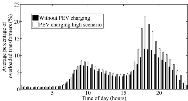
Fig. 4. Percentage of overloaded transformers for the suburban network.
