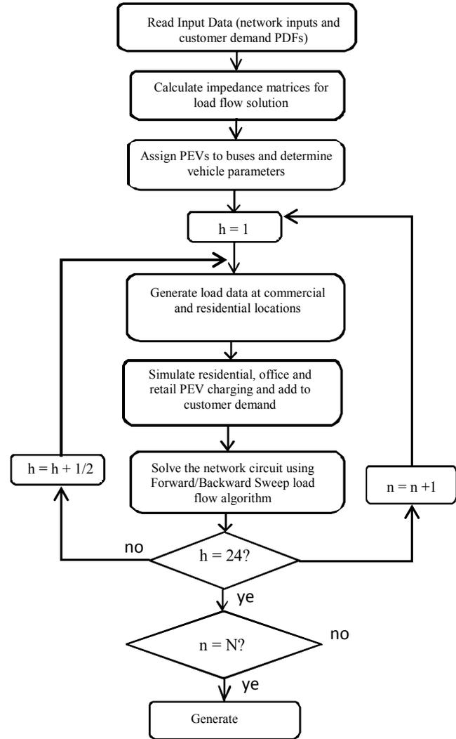
Fig. 1. MCS algorithm flow chart (h, hours; n, iterations)
