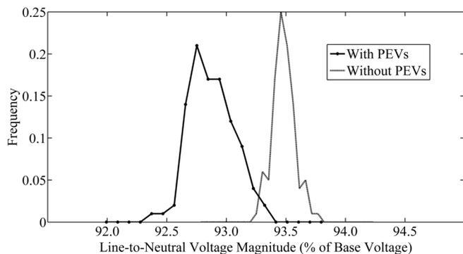
Fig. 5. Bus voltage distribution for lowest single phase bus voltage on the rural network at 18:00 hours without PEV charging and PEV charging in the high scenario.
