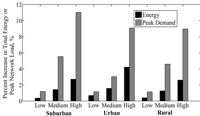
Fig. 3. Percentage increases in energy and peak load for each network in the low, medium and high scenarios
