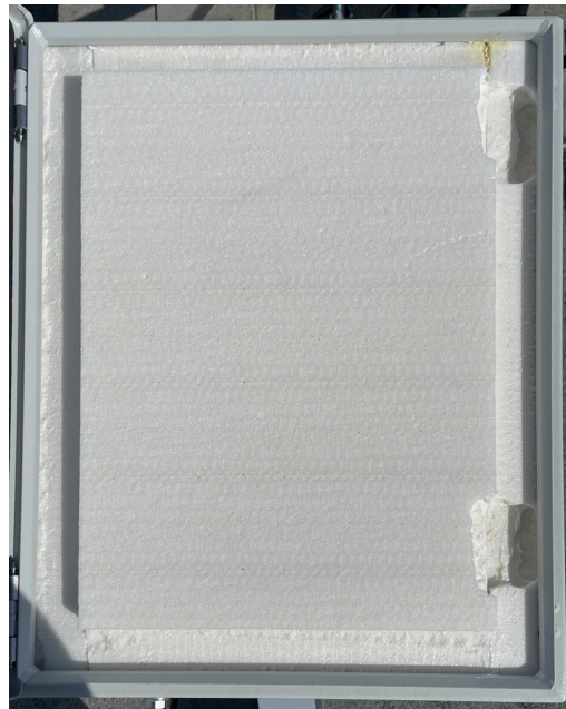
(c) The completed foam insert, fully enclosing the thermally stabilized signal chain.
