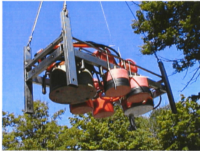
Figure 3.3 Measurement frame with transducer array (view from the bottom) (Figure courtesy of J. Tegowski)
