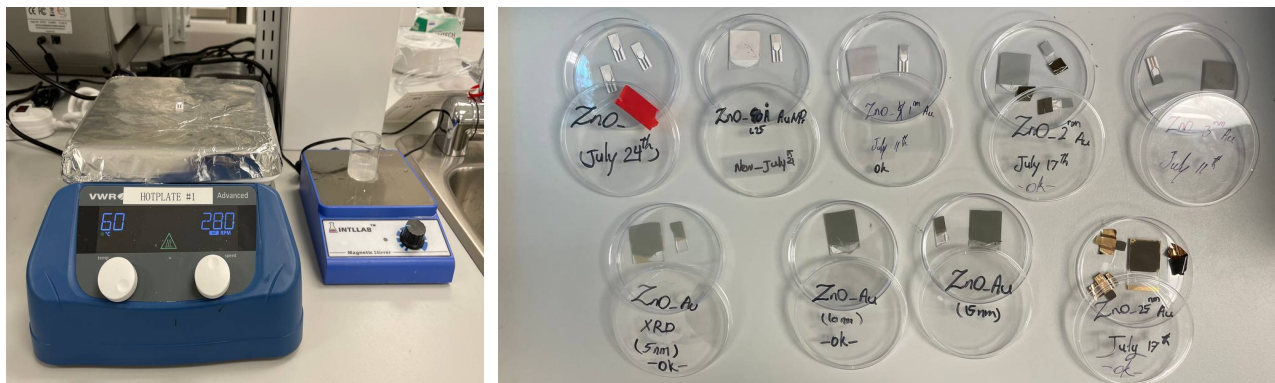
Figure 3-2-a- Deposited sensing materials onto the IDE, b-coated ZnO-based sensor with different thicknesses of Au NPs.
