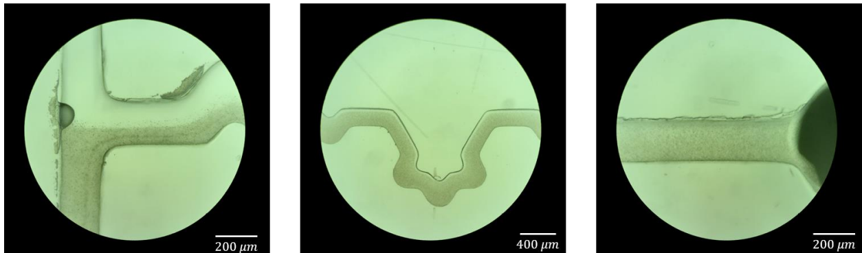
Figure 21 - Mixing in RCSM design at 1 \mu\text{l}/\text{min}
