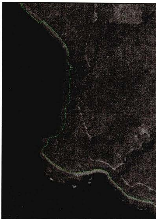
Figure 4.44 – KFA-1000. Shoreline (in green) detected in 2.7 s using Gaussian 3x3 – Roberts – Negate – 10 points.
