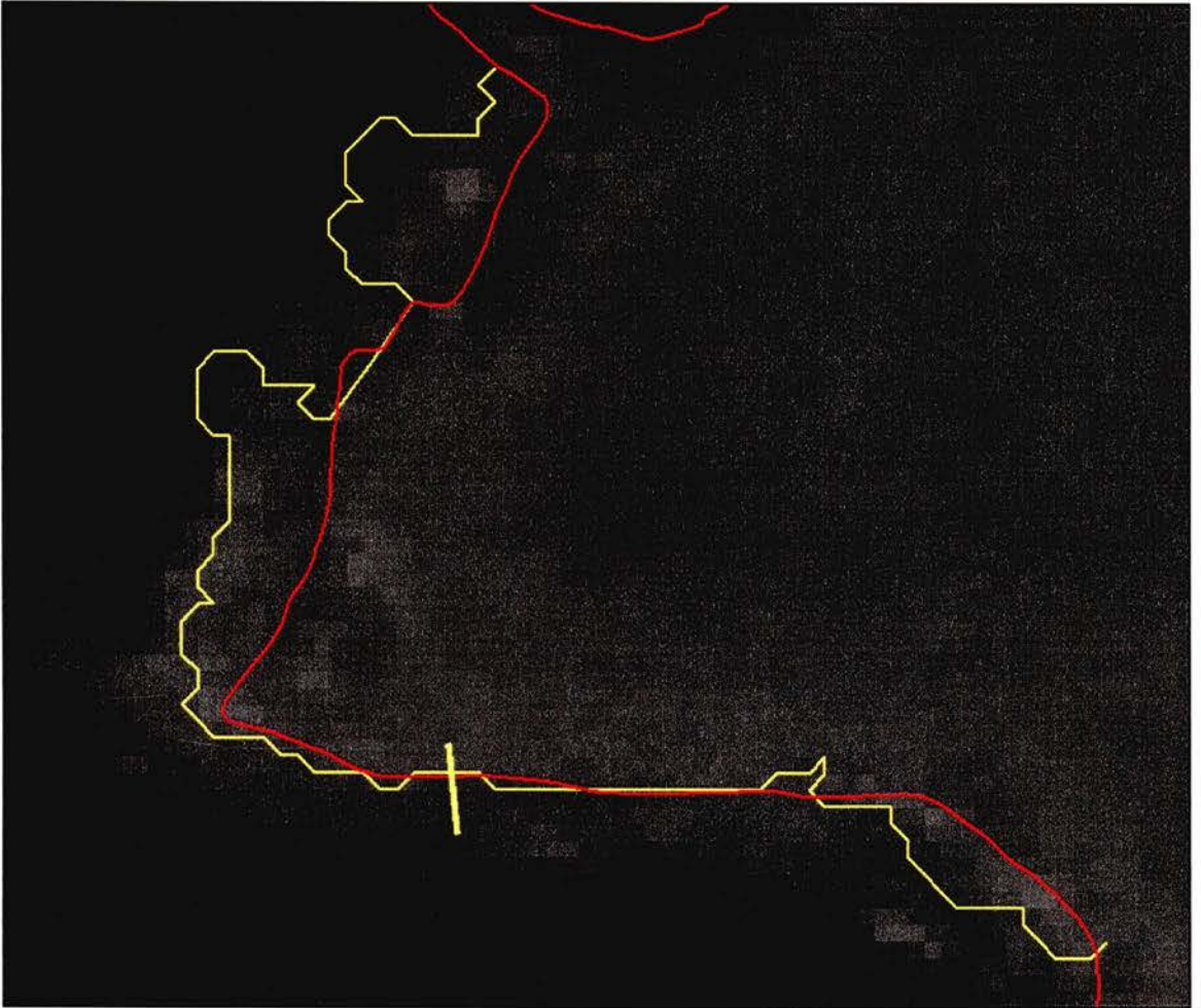
Figure 4.34 – SPOT 1 (20 m). Vector comparison. TRIM vectors are in red and the shoreline extracted by the tracing algorithm is in yellow. Shoreline profile (in yellow) is perpendicular to the shoreline.
