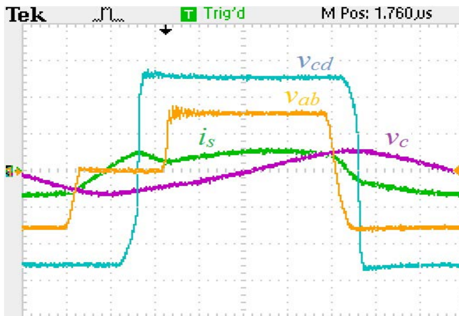
Figure 2.41 Experimental waveforms for DBSRC in discharging mode at 25% load with V_i = 64 V and V_o = 104 V. primary voltage v_{ab} (40V/div), secondary voltage v_{cd} (40V/div), resonant capacitor voltage v_c (40V/div), tank current i_s (2.5A/div).
