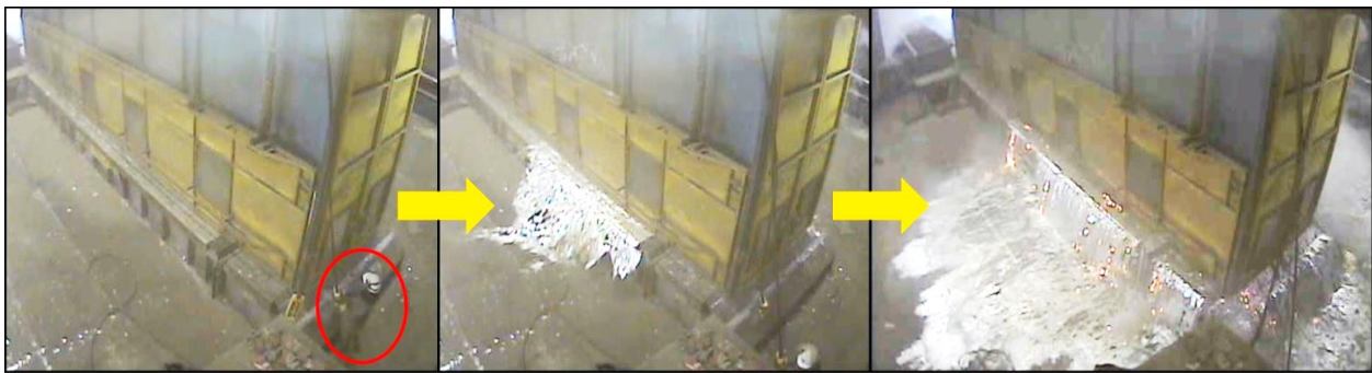
Figure 1.2. Hazard to personnel and equipment caused by insufficient venting and drainage
