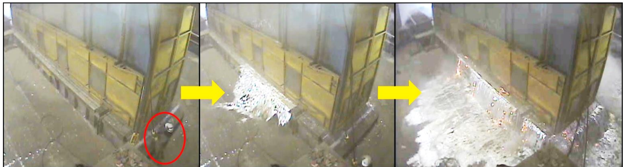
Figure 2.1. Hazard to personnel and equipment caused by insufficient venting in steel component
