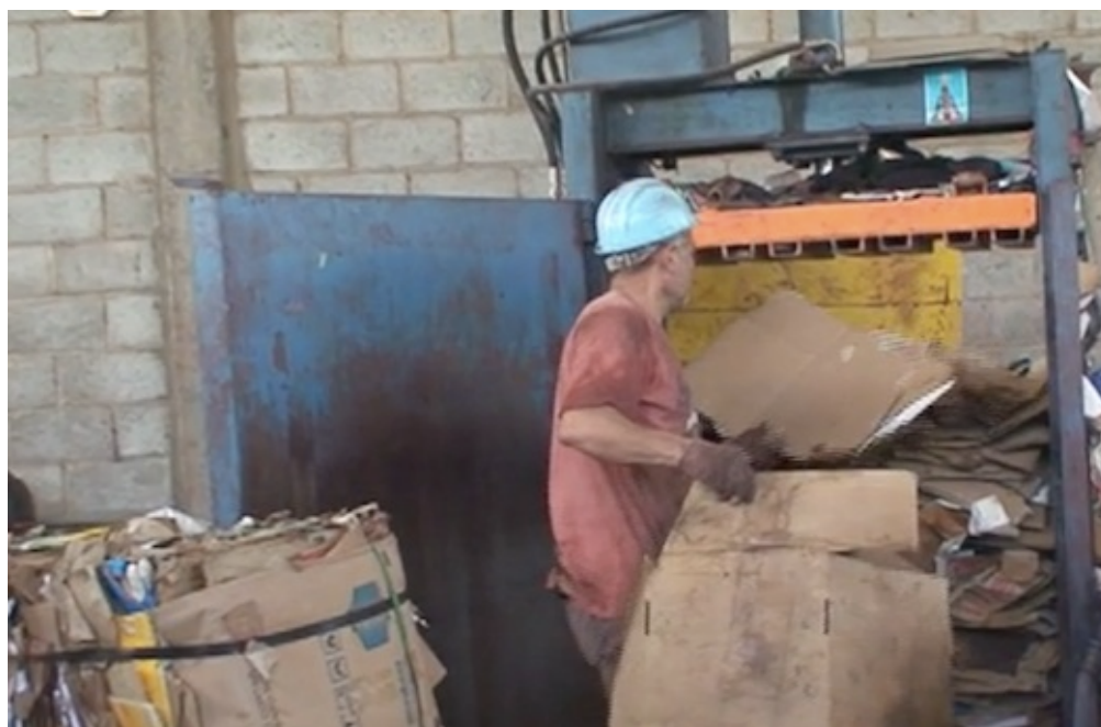
FIGURE 10. Making bales of pressed cardboard in the hydraulic press.
