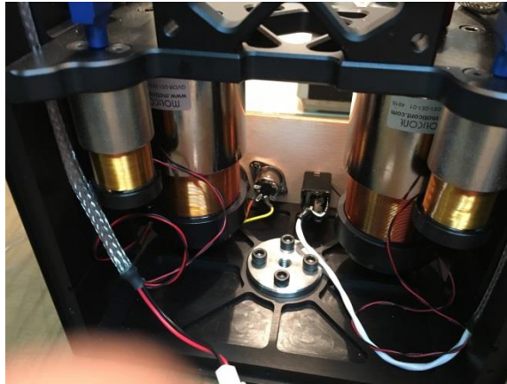
Figure 63. Final assembly, voice coil actuators and connector bulkhead.
