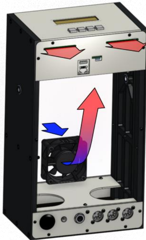
Figure 57. 3D model of enclosure with airflow path.
