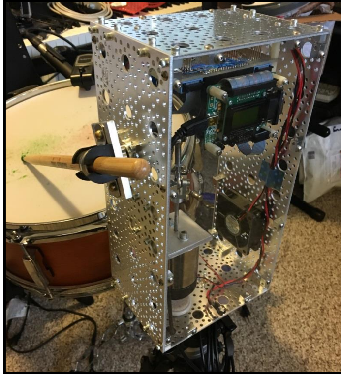
Figure 50. First integrated prototype showing VCA and electronics.
