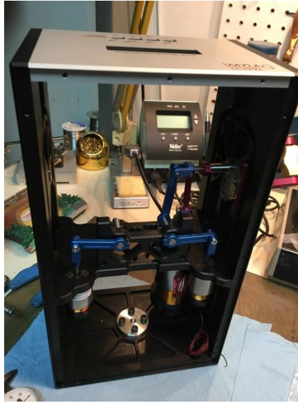
Figure 60. Final assembly, voice coils and linkages.
