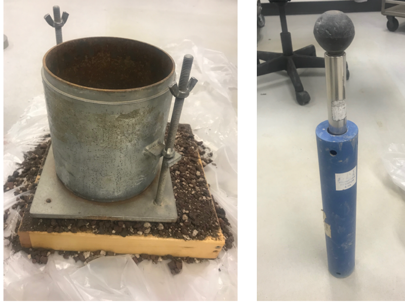
Figure A2 Cylindrical Mold and Compaction Rammer
