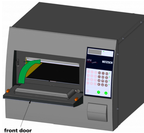
Figure A3 Heat Flow Meter
