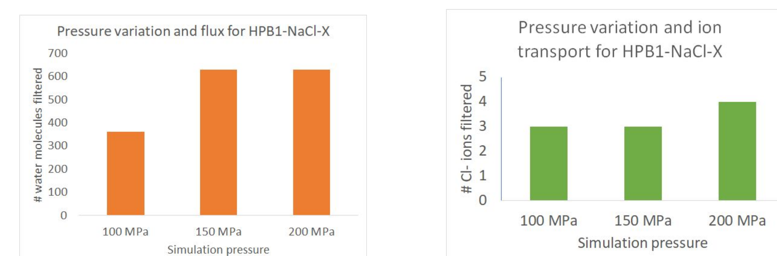
Fig. 5. Flux and salt rejection with varying pressure. Complete rejection of sodium. Out of 95 chloride ions in solution, only a maximum of four are transported through the membrane.
