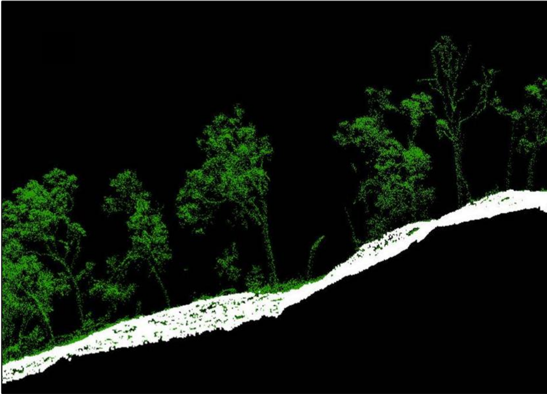
Figure 12: A vertical cross section plane of a lidar point cloud acquired from a hilly Acacia koa woodland in Hawaii in February of 2010. The white points are the last return. The lidar was flown on a Jet Ranger helicopter at approximately 685m altitude. The emitted light had a wavelength of 1064nm. The pulse rate was 260 KHz, and the spatial footprint was approximately 14cm [41].
