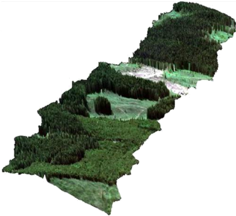
Figure 4: Image from UVic's Specim AISA (airborne imaging spectrometer for applications) sensor draped over a lidar digital surface model. Colour composite is Red: 640nm, Green: 550nm and Blue: 460nm.
