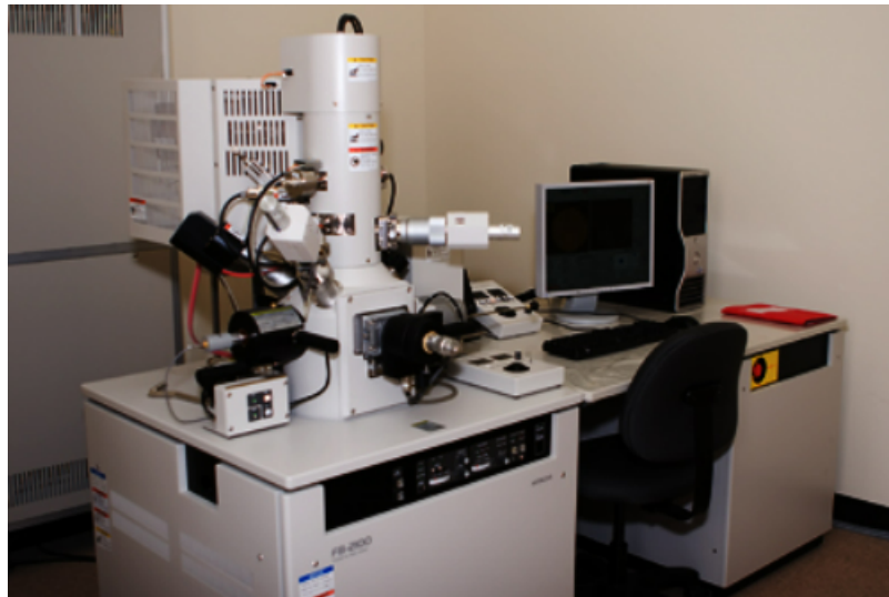
Figure 8 - Hitachi FB-2100 Gallium focused ion beam machine in the Advanced Microscope Facilities at the University of Victoria.
