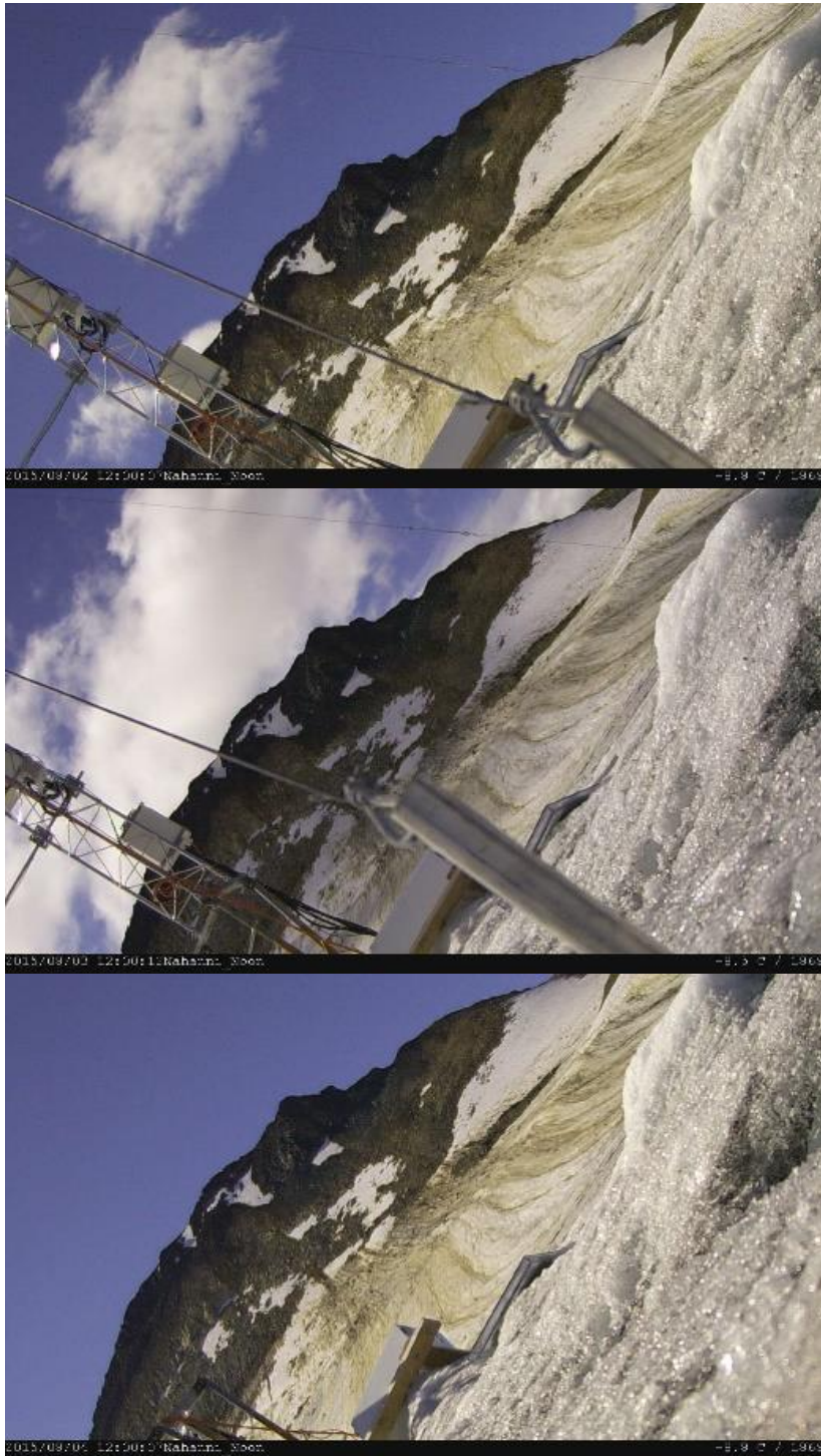
Figure 6: Image of the meteorological tower toppling over in summer 2015, from top to bottom: 08/02, 08/03, 08/04. The camera is located on the tripod which toppled one month prior. The guy wire anchor can be seen coming out in the second picture.
