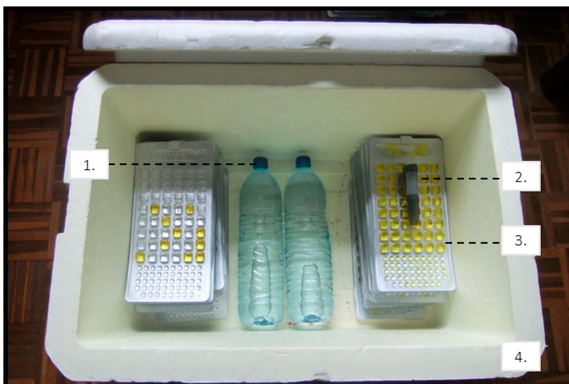
Figure 1. The expanded polystyrene (EPS) incubator with Colilert trays and 1.5 L polystyrene bottles with heated water. Labels: 1. Polystyrene bottles, filled with water; 2. Temperature data logger; 3. Colilert trays; 4. EPS foam cooler.
