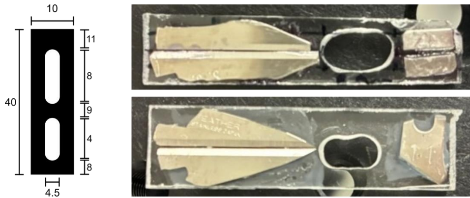
Figure 3.9. Image of slits used for free-space coupling into spectrometer. (left) Dimensions for the acrylic pieces shown on the right, units in millimeters, (right, top) 105 \mu\text{m} slit, (right, bottom) 200 \mu\text{m} slit.
