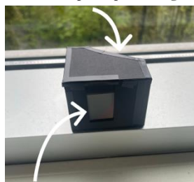
Figure 1.6. Images of a simple spectroscope which can be built at home 105 .
