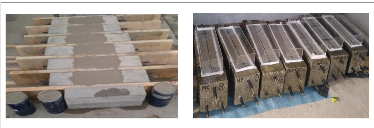
Figure D9.1 Casting of repair material Mix P
