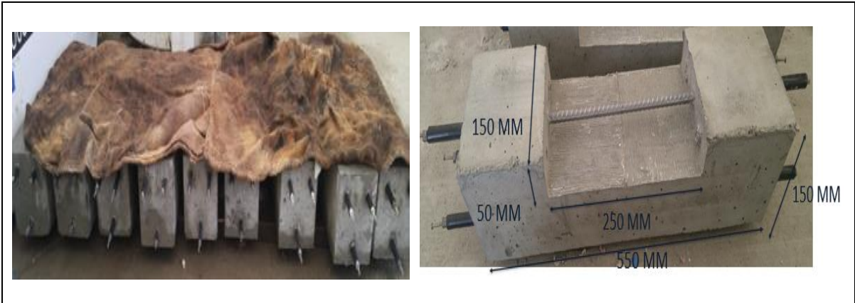
Figure D5.1 Curing of specimens
