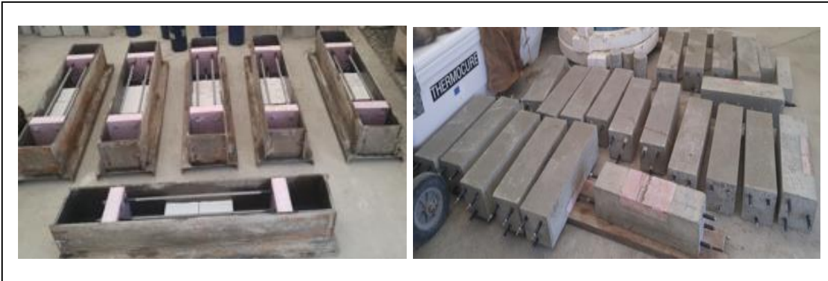
Figure D3.1 Molding preparation of specimens
