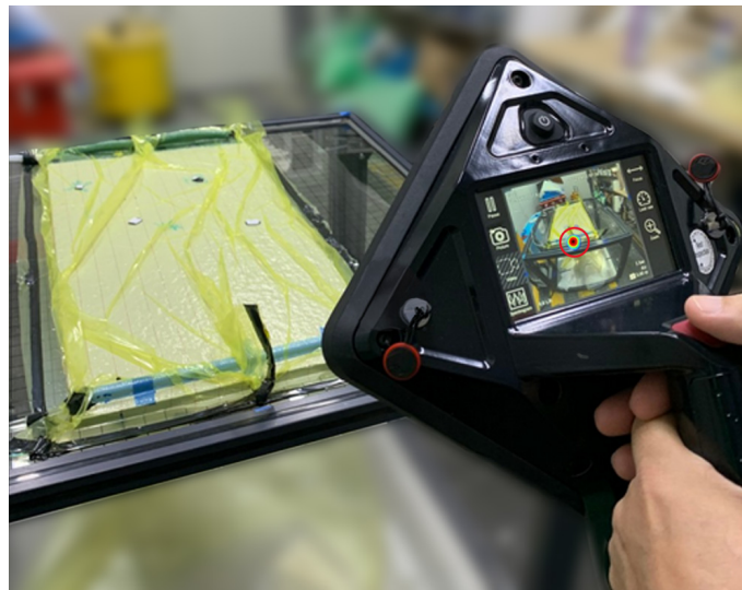
Figure 2.12: Ultra CE; an advanced ultrasound leak detector using 124 microphones, detecting leaks in quiet environments [37]
