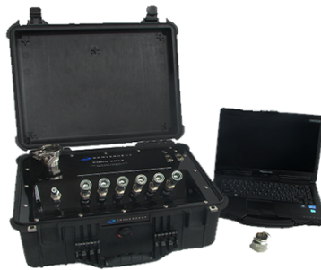
Figure 3.4: COHO 601 flowrate measurement setup
