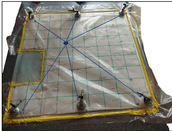
Figure 3.29: Cost function calculation for a single leak for vacuum ports configuration in corners
