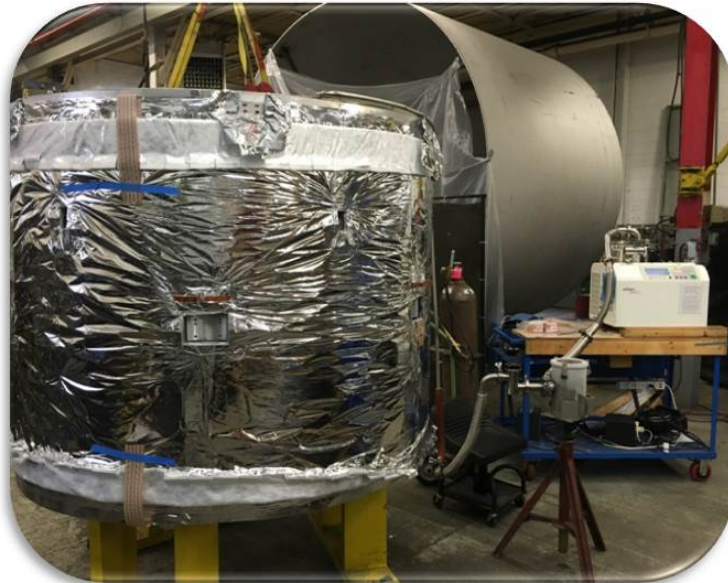
Figure 2.10: Helium gas leakage detector hood technique used on a vacuum bag; a large area could be covered with this method [29]
