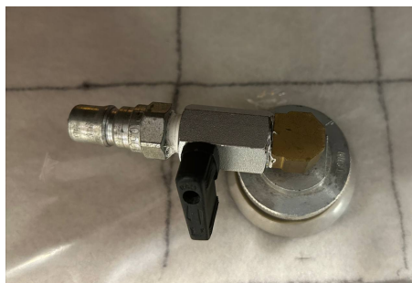
Figure 3.2: Vacuum connector or port which connects the layup to the vacuum system; the valve could be used to disconnect the system
