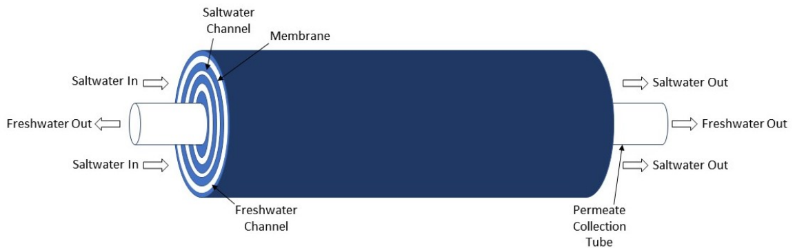
Figure 4.4: Spiral wound membrane module.
