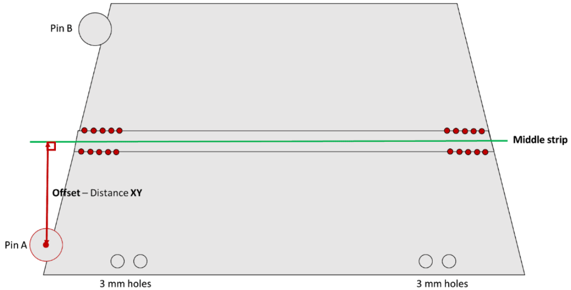
Figure 6.1: A diagram showing how the offset measurement was taken at Triangle Labs. A 24 board is depicted in this diagram, as the alignment features are on the left 3 .
