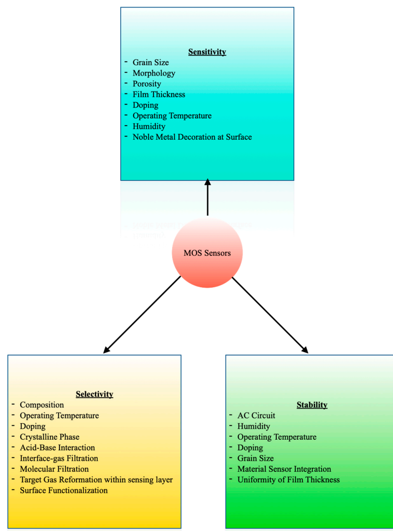
Figure 6. Parameters Affecting the Sensing Performance of MOS Sensors.
