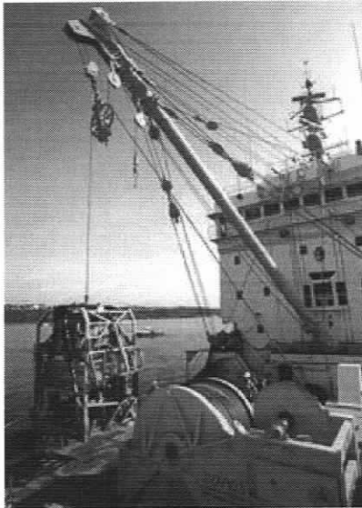
Figure 1.2 (a) : A caged ROV system being deployed off the ship. The cage or garage bearing the ROV is linked to the ship through an armored tether and is used to position the ROV. The ROV umbilical links the ROV to the cage, both of which are underwater.
