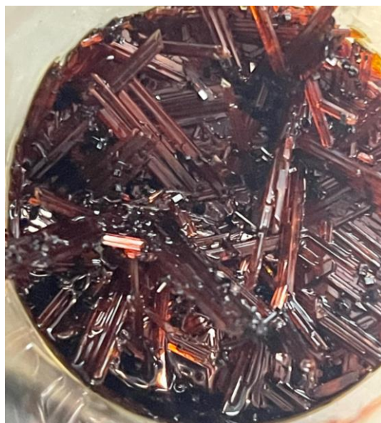
Figure 2.17: Cobalt carbonyl crystals that have been recrystallized and isolated from hexanes.
