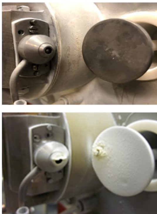
Figure 1.4: Baffle cone (top) before and Bottom after running methylalumoxane.
