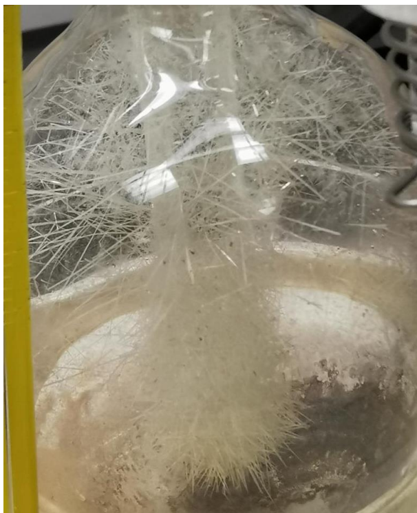
Figure 2.6: Sublimation of \text{Cl}_3\text{SiCo}(\text{CO})_4 in a Schlenk flask contained initially in a \text{N}_2 atmosphere. Sublimation was completed over 2 h with static vacuum, a cold finger with cold water, and an oil bath held to 40^\circ\text{C} .
