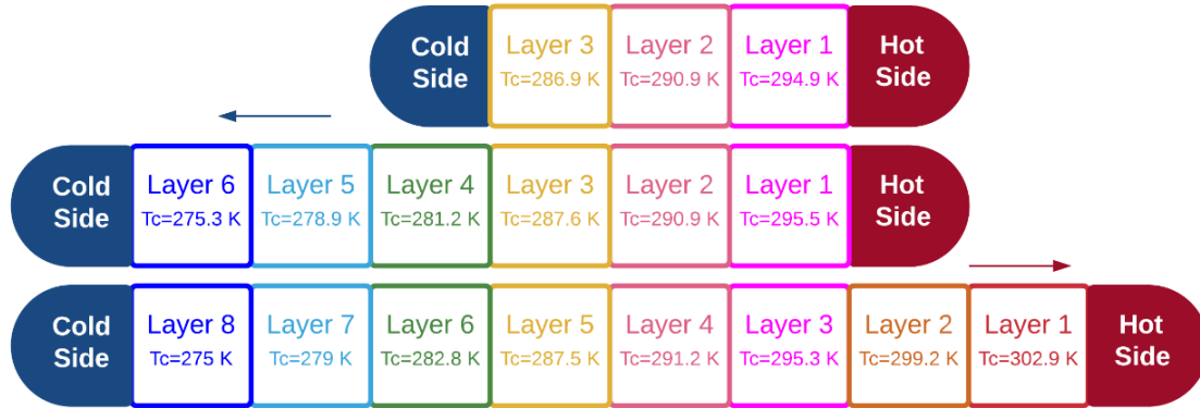
Fig.30 FOM multilayer regenerators: Layer composition for the FOM regenerators, which the reference transition temperature presented is characterized via DSC measurements considering a heating protocol.
