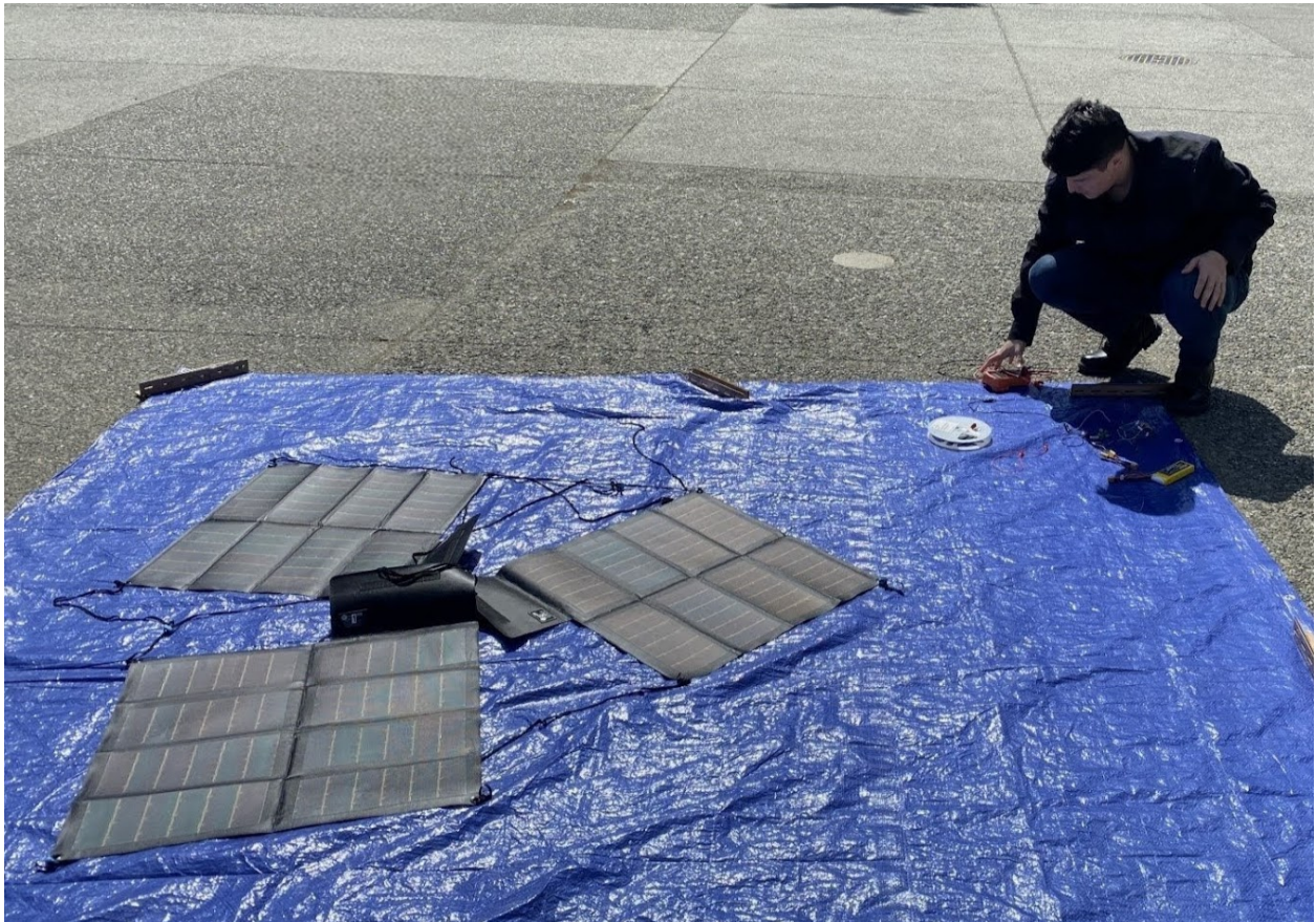
Figure 3.4: Outdoor testing of the custom battery charging circuit with the flexible solar panels that will be used on ALTAIR.
