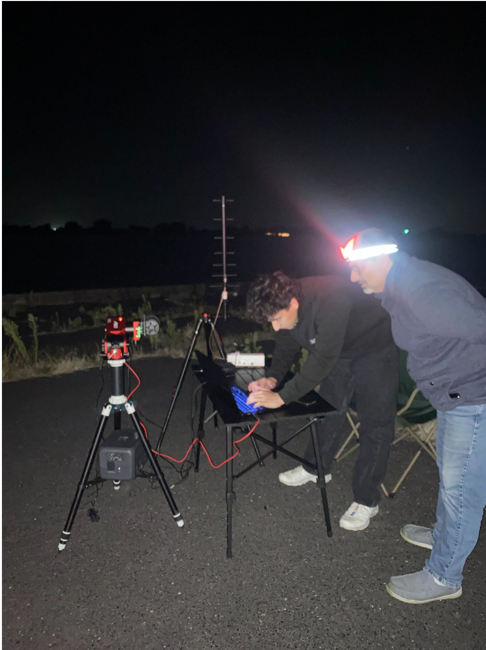
Figure 3.13: The portable ALTAIR ground station during a field test conducted by the McGill engineering team. The system will allow for complete monitoring and control of the airborne payload.
