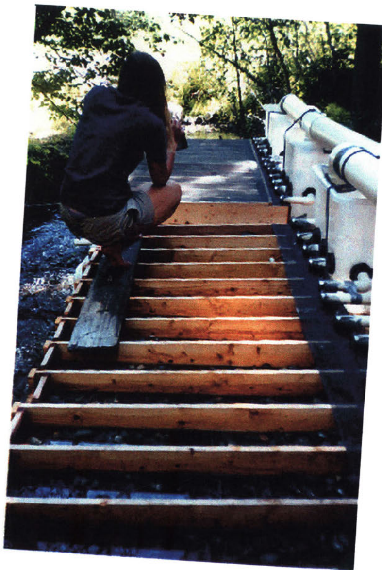
Figure 4. Artificial stream channels (side view), showing header boxes, outflow pipes, mesh screens, and 24 experimental channels (photo by L. Shama).
