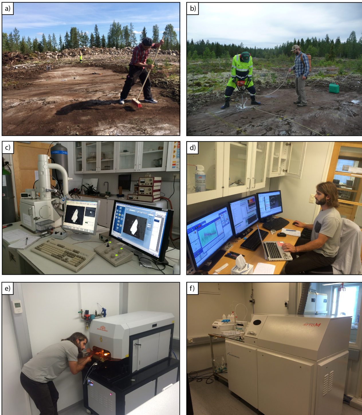
Figure 1-4 Methods of investigation. a) Cleaning and exposing transects, featuring Sayab Muhammad; b) Operating the hand held drill, featuring Tuomo Turinen; c) Locating monazites on the SEM using EDS methods at the GTK headquarters; d) Operating the LA-ICP-MS system at the GTK headquarters; e) The laser ablation machine by Photon-Machine at the GTK headquarters; f) The ATTOM mass spectrometer machine by Nu-Instruments at the GTK headquarters.
