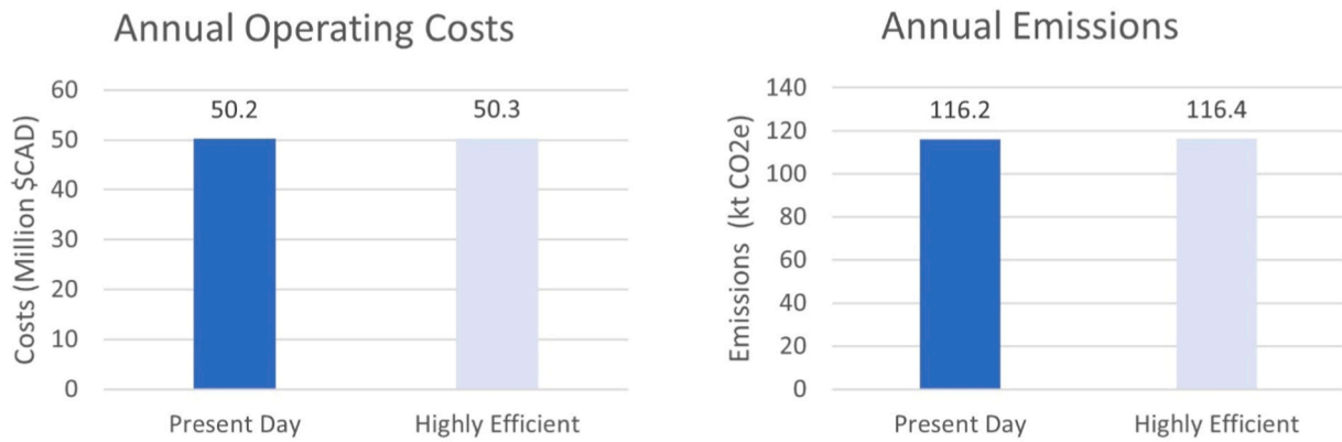
Fig. 9. Annual operating costs and annual emissions for the present day and highly efficient building stocks before the enactment of demand response strategies.
