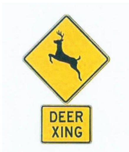
Figure 4.7 Deer crossing sign with symbol and educational plaque (Source: National Joint Committee on Uniform Traffic Control Devices and American Association of State Highway Officials (1971))
