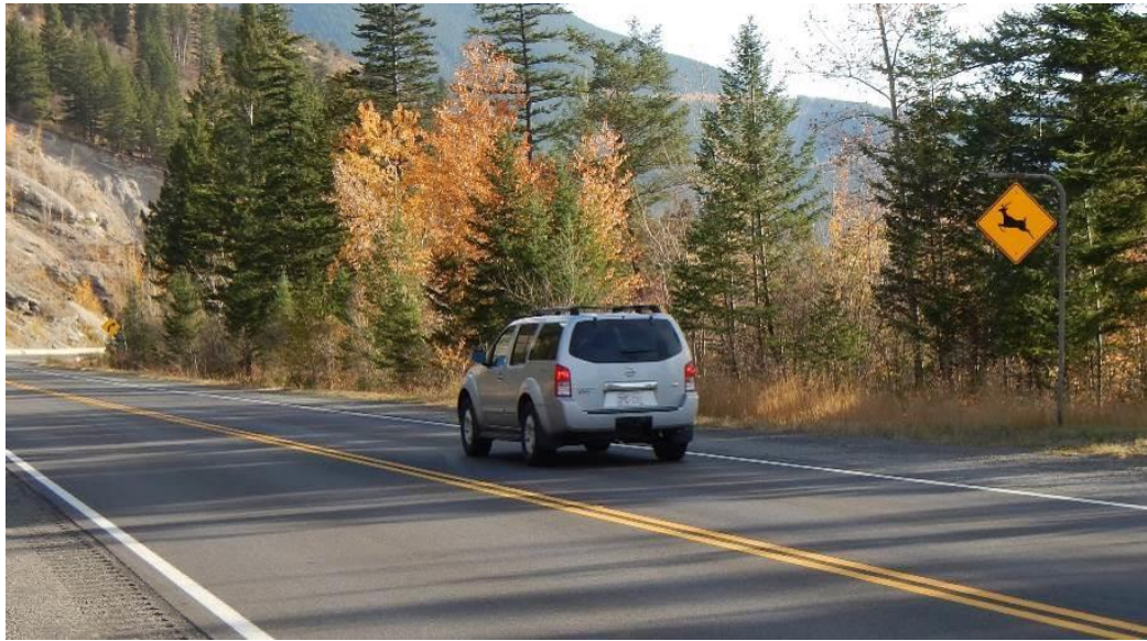
Figure 6.13 Vehicle with unimpeded headway
