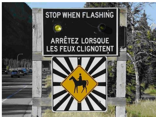
Flashing lights and patterned border
