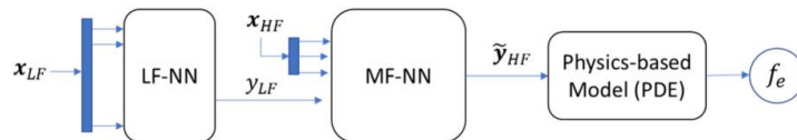
Fig. 2.4 Architecture of MF-PINN. Samples are selected using a design of experiments method such as Latin hypercube sampling[18]
