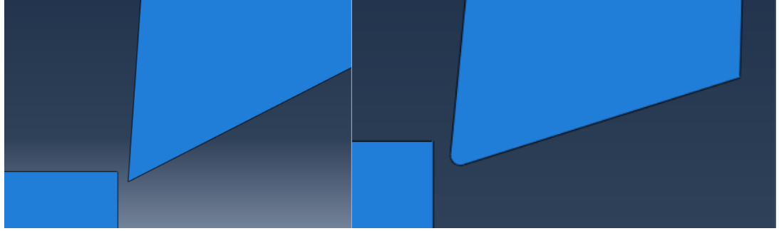
Fig. 3.8 Sharp (left) and round (right) tool edges
