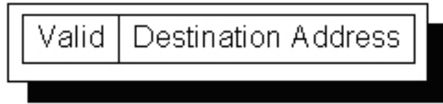
Figure 2.11: Indirection Buffer Structure
