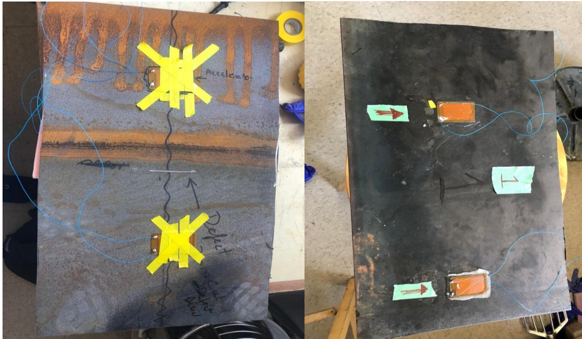
Figure A.2.1: Steel plate as a Specimen
