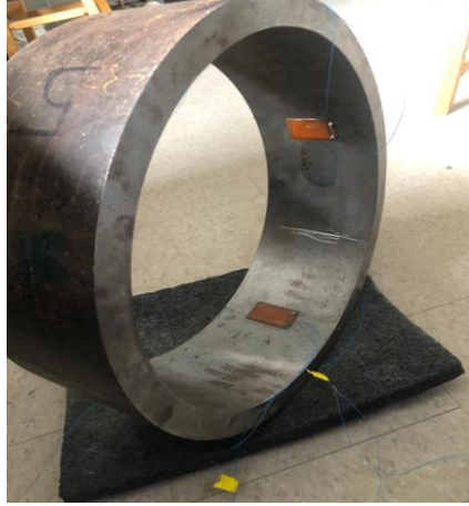
Figure A.1.1: Steel ring with Piezo Patches
