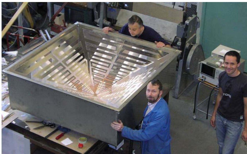
Figure 1.7: The Eleven feed built for 150 - 1500 MHz observations at the Green Bank radio telescope [11].
