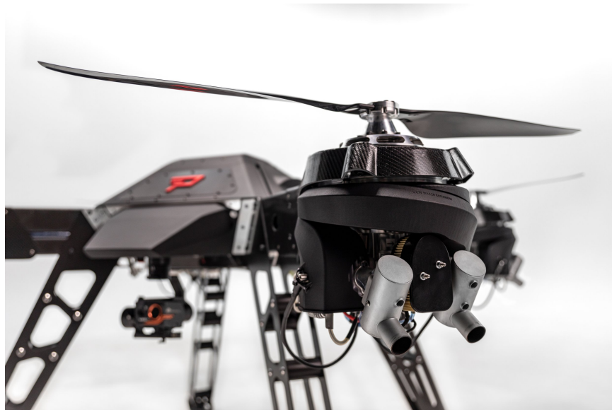
Figure 4: Parallel Flight Technologies UAS power unit located in each boom [16]
