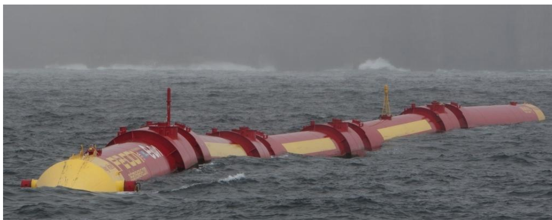
Figure 1.3: The P2 Pelamis is an attenuator made up of five connected bodies totaling 180m in length and 4m in diameter. Each of the WEC's joints contain a power take-off to convert the bodies relative motion into electricity( www.pelamiswave.com ).
