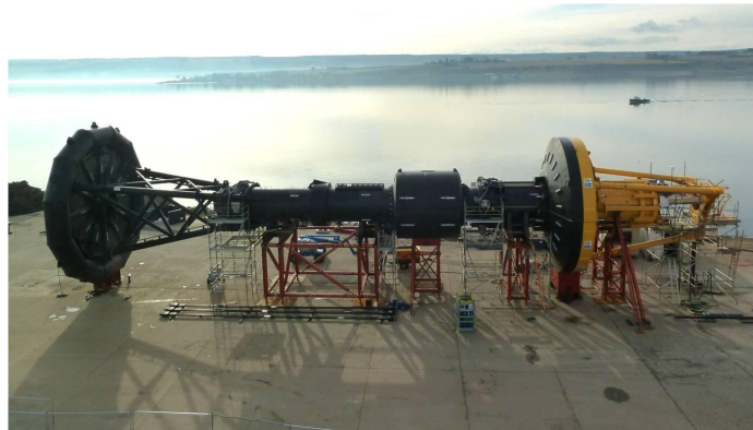
Figure 1.6: Ocean Power Technologies' P150 PowerBuoy is self-reacting point-absorber rated at a capacity of 150kW. The device is shown horizontally prior to installation off Scotland's northeast coast in 2011 ( www.oceanpowertechnologies.com ).
