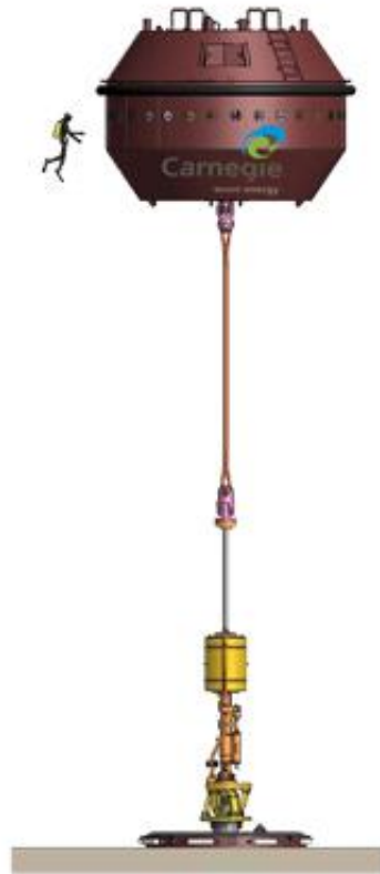
Figure 1.5: Carnegie's CETO III is a one-bodied point absorber located off the shores of Garden Island in Western Australia ( www.carnegiewave.com ).
