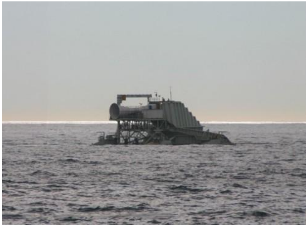
Figure 1.4: The OceanLinx MK1 was a 500 tonne oscillating water column WEC installed in Port Kembla, Australia, in 2005( www.oceanlinx.com ).
