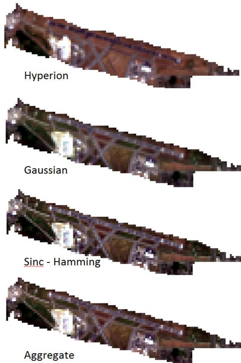
Figure 4.14: True colour images showing the visual differences between the EO-1 Hyperion sensor imagery (July 2013), EnMap simulated from airborne data (July, 2014) using different modelled PSFs. Map scale is roughly 1:35,000.
