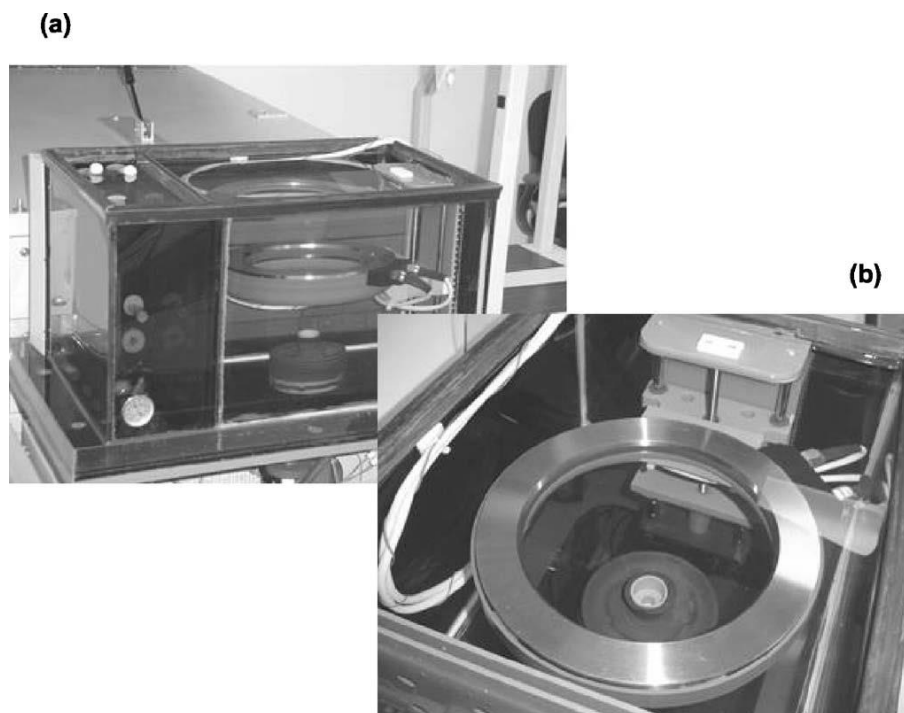
Figure 5: Karmanos CURE system showing the tank (a), and the transducer ring (b) [1].
