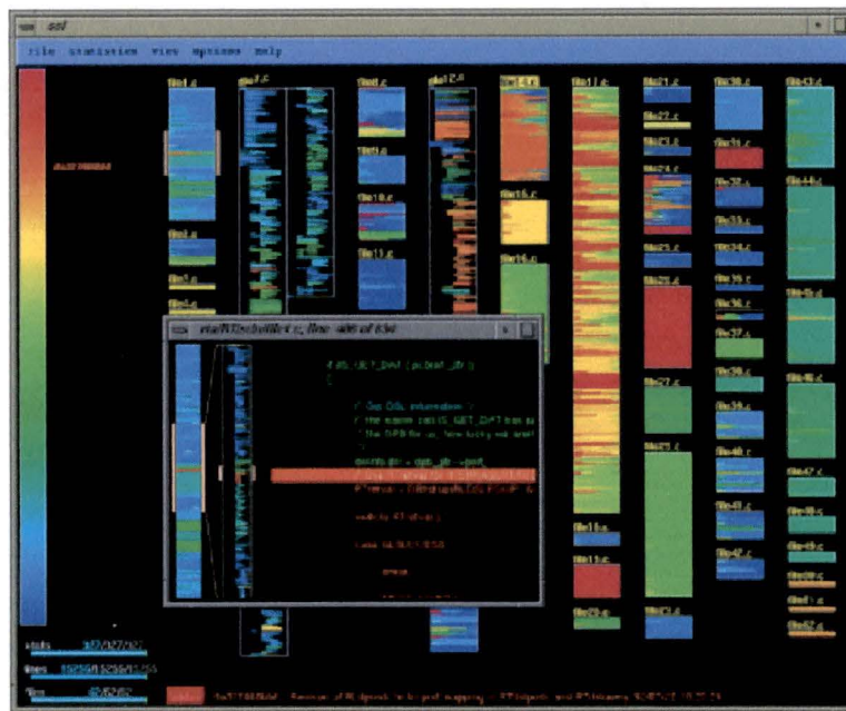
Figure 2.2: A screenshot of SeeSoft, showing the age of code. The newest lines are in red, and the oldest are in blue, with a rainbow color scale in between.
